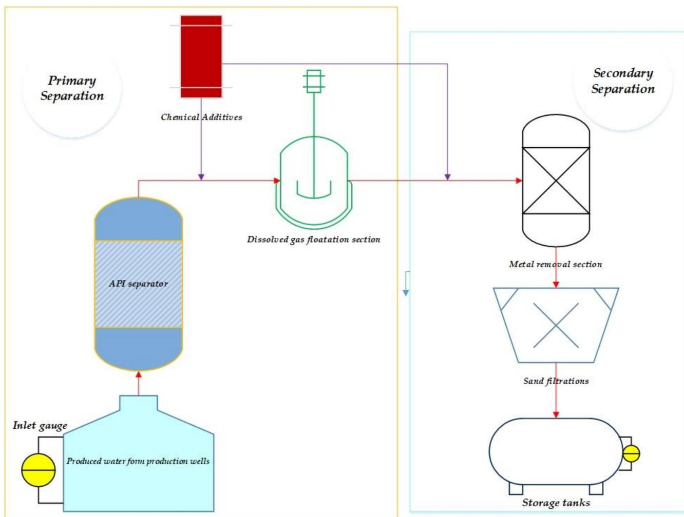
**Figure 1.** PFF method to retreat produced water.
