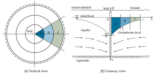
**Figure 6.** Formation of cone of depression of groundwater level during pumping. Q is the water yield of the pumping well,  $[L^{3}T^{-1}]$ .
