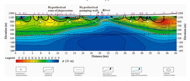
**Figure 5.** Schematic flow lines of a practical site according to the distribution of apparent resistivity, with a hypothetical pumping well added (modified from [27]).
