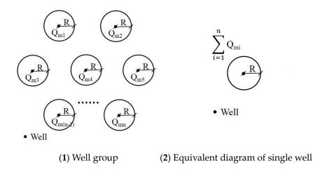
**Figure 4.** Influence radius in well group pumping and single well pumping in influence radius theory. R is the influence radius, [L];  $Q_{mi}$  is the maximum water yield of pumping well i, [L<sup>3</sup>T<sup>-1</sup>]; and n is the number of pumping wells.
