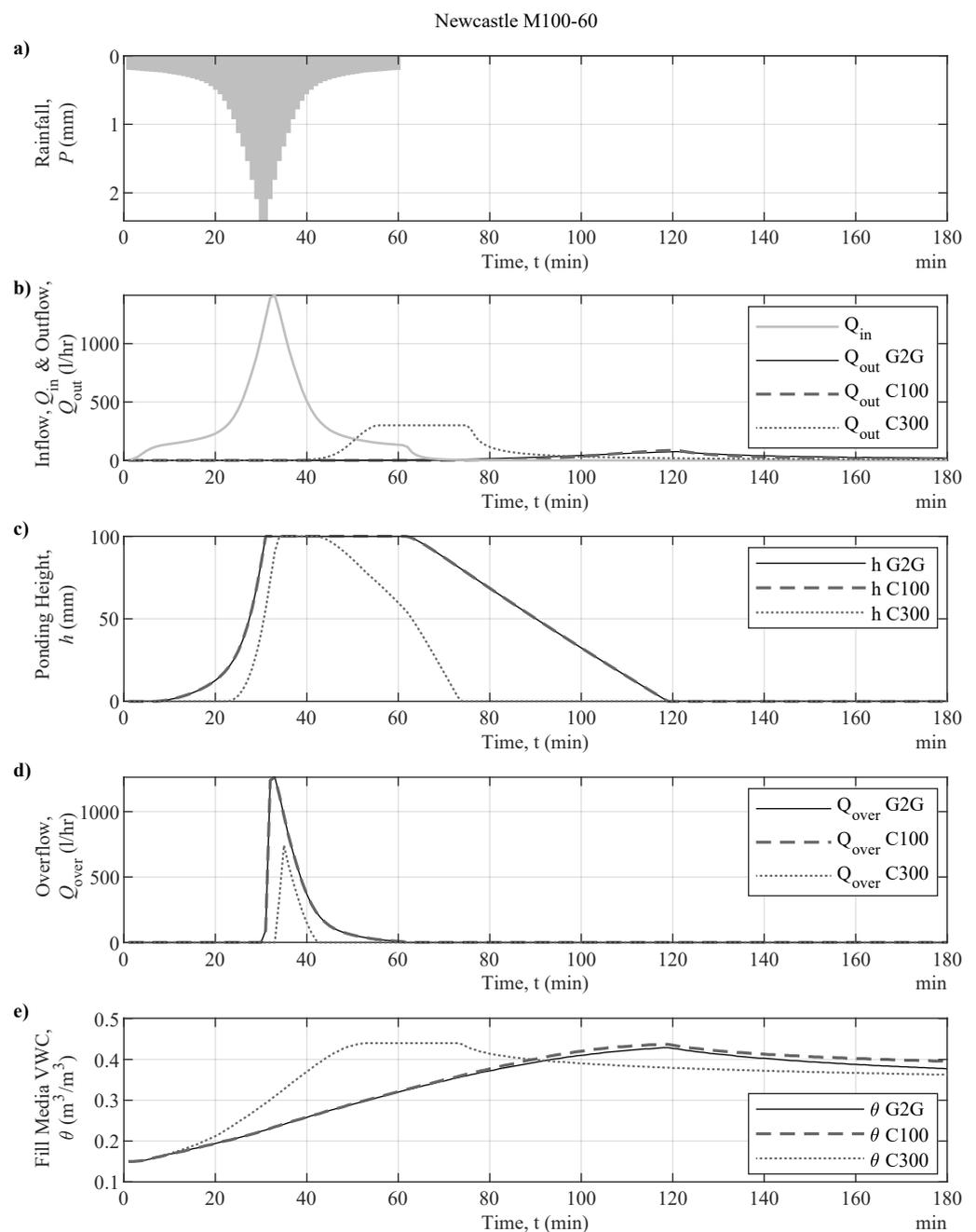
**Figure A2.** Modelled hydraulic response of bioretention systems in response to a 100-year return period 60-min duration storm event for Newcastle, UK. (a) Rainfall depth; (b) system inflow and outflow; (c) ponding height; (d) overflow; and (e) volumetric water content (VWC) of the fill media.
