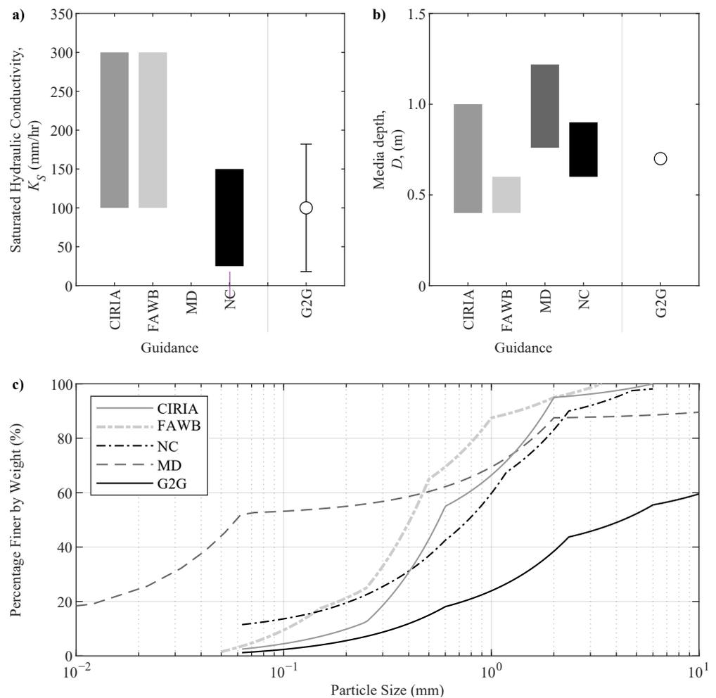
**Figure 3.** Comparison of G2G and Guidance Document ranges for: (a) Saturated Hydraulic Conductivity, with G2G plotted as mean  $\pm 1$  standard deviation; (b) media depth, with G2G plotted as a single value; and (c) particle size distribution (plotted at the middle of the allowable range; linear interpolation of data is presented on the logarithmic  $x$ -axis).
