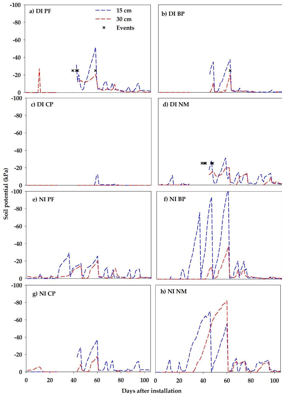
**Figure 3.** Daily average soil matric potential (09:00 am) at 15 and 30 cm deep in tomato plots during 2019 field experiment under drip irrigation (DI) treatment with (a) landscape fabric mulch (DI PF), (b) black plastic mulch (DI BP), (c) clear plastic mulch (DI CP), (d) no mulch (DI NM), and no irrigation treatment (NI) with (e) landscape fabric mulch (NI PF), (f) black plastic mulch (NI BP), (g) clear plastic mulch (NI CP), and (h) no mulch (NI NM).
