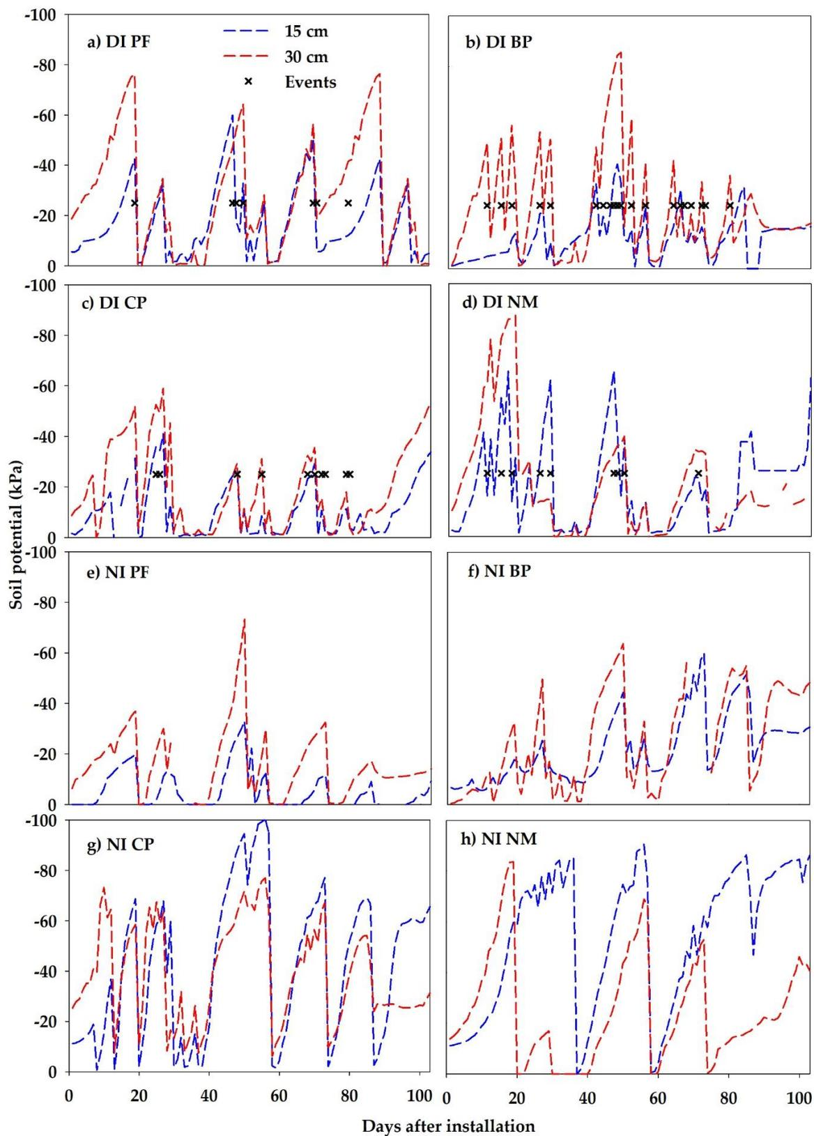
**Figure 4.** Daily average soil matric potential (09:00 am) at 15 and 30 cm deep in tomato plots during 2020 field experiment under drip irrigation (DI) treatment with (a) landscape fabric mulch (DI PF), (b) black plastic mulch (DI BP), (c) clear plastic mulch (DI CP), (d) no mulch (DI NM), and no irrigation treatment (NI) with (e) landscape fabric mulch (NI PF), (f) black plastic mulch (NI BP), (g) clear plastic mulch (NI CP), and (h) no mulch (NI NM).
