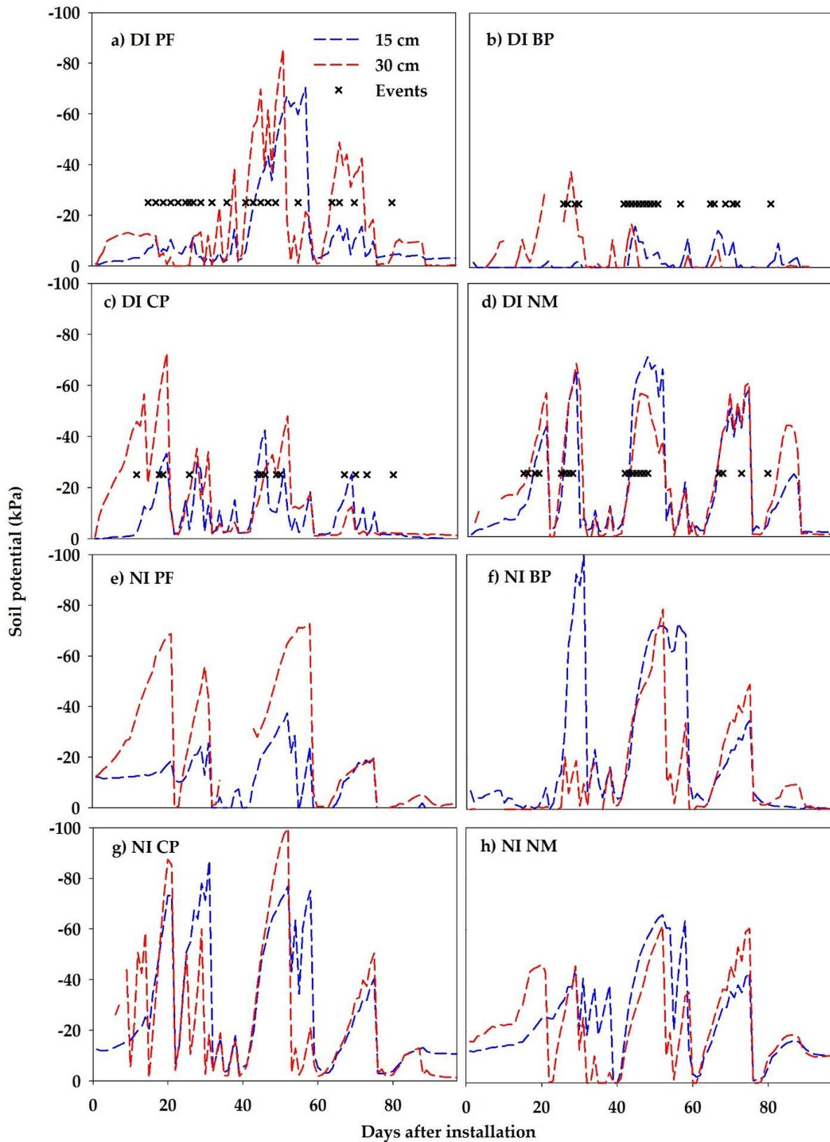
**Figure 6.** Daily average soil matric potential (08:00 am) at 15 and 30 cm deep in watermelon plots during 2019 field experiment under drip irrigation (DI) treatment with (a) landscape fabric mulch (DI PF), (b) black plastic mulch (DI BP), (c) clear plastic mulch (DI CP), (d) no mulch (DI NM), and no irrigation treatment (NI) with (e) landscape fabric mulch (NI PF), (f) black plastic mulch (NI BP), (g) clear plastic mulch (NI CP), and (h) no mulch (NI NM).
