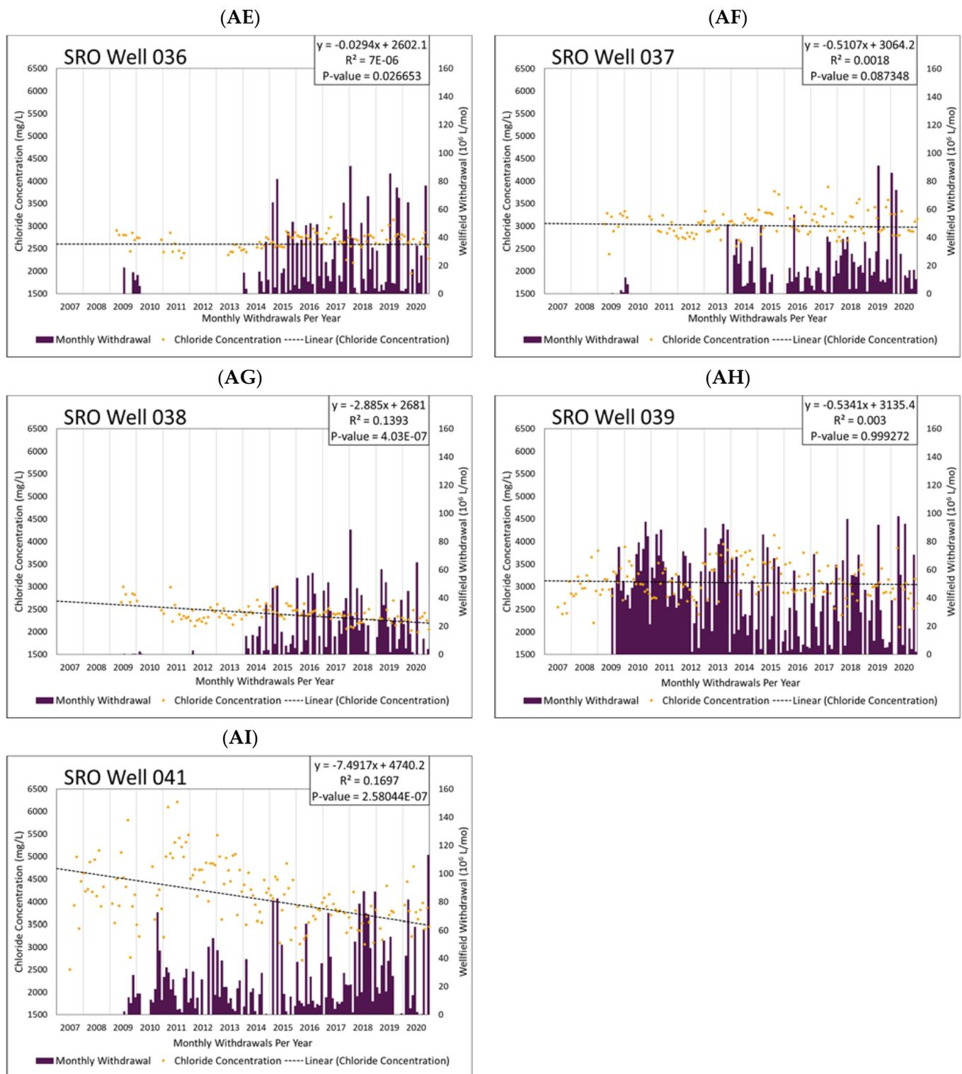
Figure 5. Plots of dissolved chloride concentration with time, monthly cumulate pumping, the calculated values of  $R^2$  and  $p$ -values and the regression equations for the trend line for Hawthorn Aquifer Zone 1 production wells.
