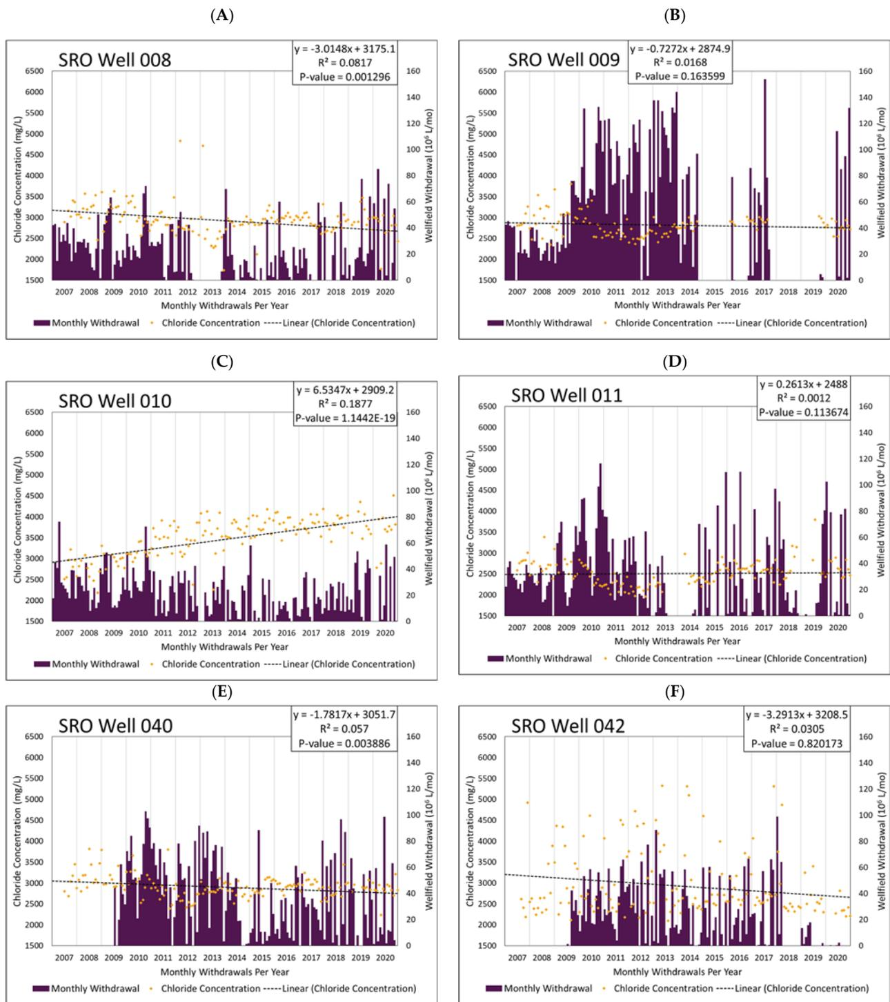
**Figure 6.** Plots of dissolved chloride concentrations with time, monthly cumulate pumping, the calculated values of  $R^2$  and  $p$ -values and the regression equations for the trend line for the Lower Hawthorn Aquifer production wells.
