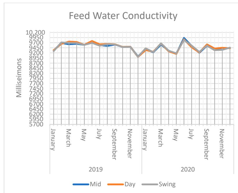
**Figure 11.** Conductivity of the feed water for 2019 and 2020. The mean is near 9400 millisiemens, which is an estimated TDS of 4700 mg/L or a dissolved chloride value of about 2585 mg/L.
