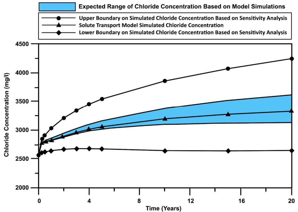
Figure 7. Original solute transport model for the South Collier County Wellfield based on a pumping rate of 41,667 m<sup>3</sup>/d (11 MGD) [32].
