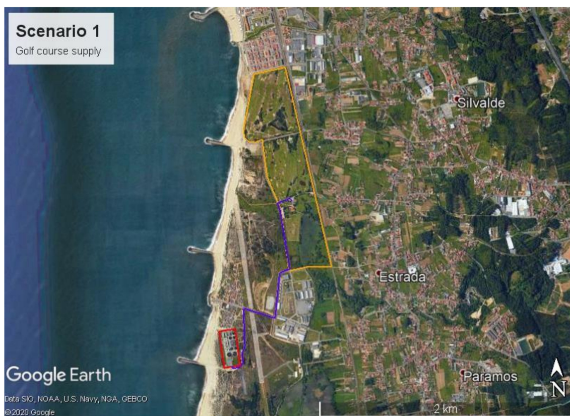
Figure 5. Scenario 1: WtR supply, provided by Espinho WWTP (in red), by pressurized network (pipe in blue) to the Oporto Golf Club bordered in orange.
