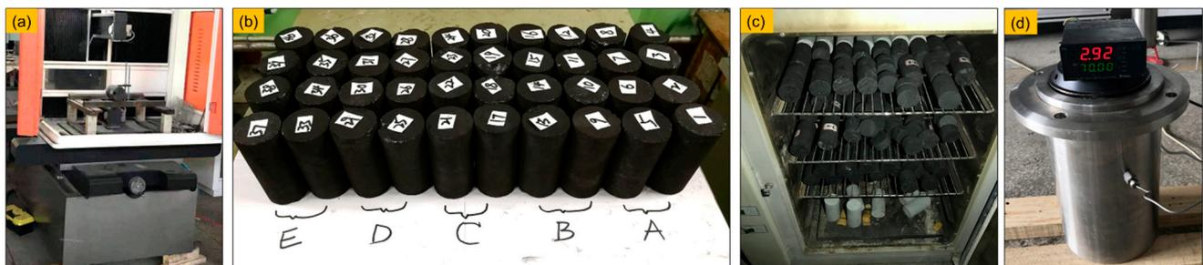
Figure 2. Sample preparation setups. (a) Line cutting machine; (b) coal samples; (c) drying oven; (d) water injection apparatus.
