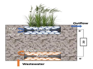
Figure 1. Schematic of constructed wetland MFC (CW-MFC) setup (R: Resistance).
