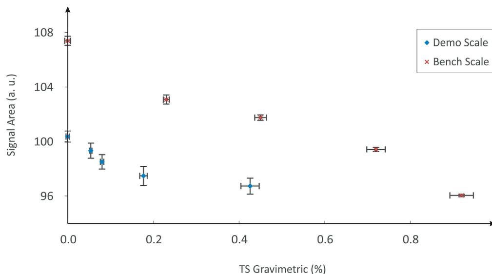
**Figure 3.** Correlation between the sensor signal and gravimetric analysis obtained during the bench-scale and the demo-scale tests. The error bars are defined as the standard deviation of the sensor signals (vertical error bars) and the standard error calculated from the gravimetric analysis triplicates (horizontal error bars).
