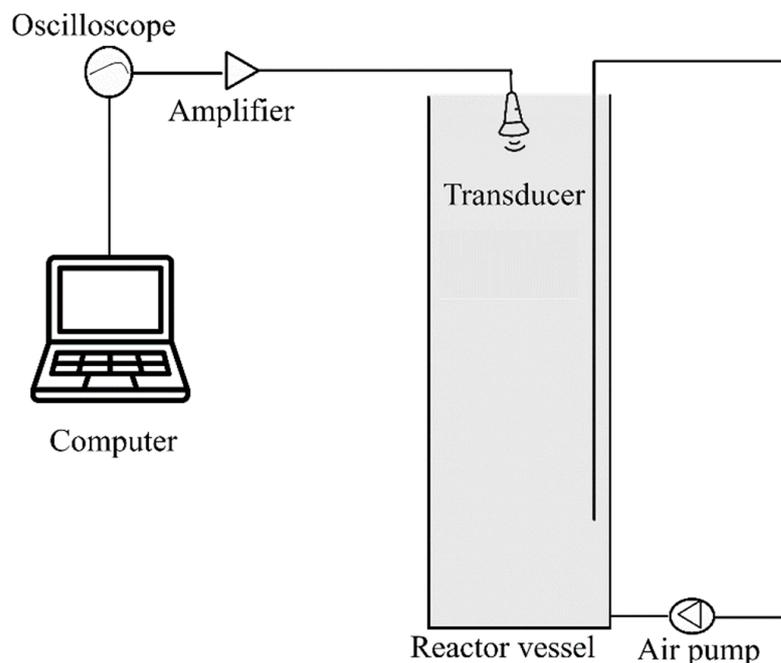
**Figure 1.** Setup used for the bench-scale experiments.
