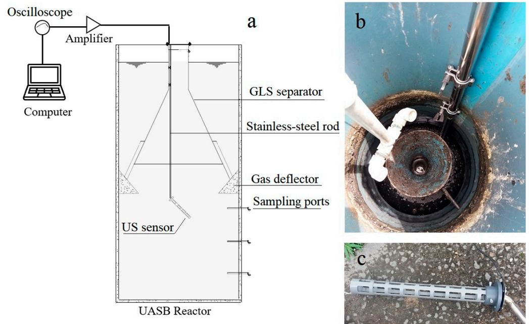
**Figure 2.** Setup used for the demo-scale experiments. (a) Cross-section of the UASB reactor showing the position where the sensor was installed. (b) Top view picture of the UASB reactor, which shows the stainless still support used to fixate the sensor. (c) Photo of the sensor housing before it was inserted in the reactor.
