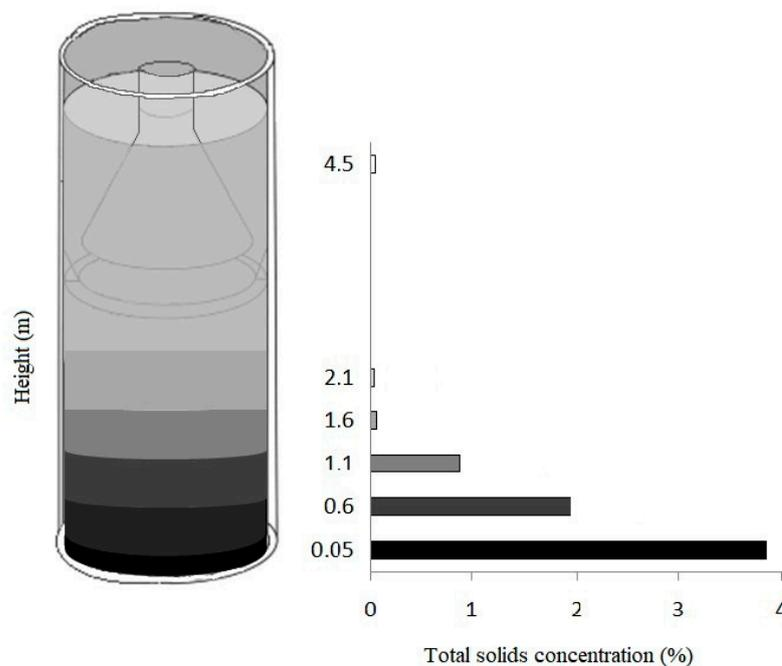
**Figure 4.** Solids profile inside the demo-scale UASB reactor obtained by gravimetric analysis.
