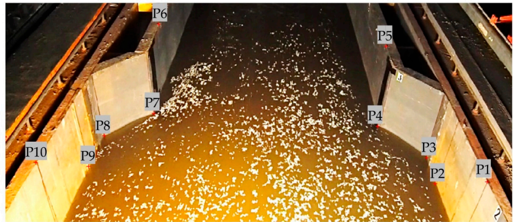
Figure 2. Locations of GRPs for 0.75 contraction ratio. The locations are designated as P1 through P10.
