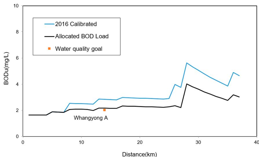
**Figure 7.** Water quality distribution in the Whangyonggang River after WLA application according to the fuzzy model. The allocated BOD load is the water quality distribution in the Whangyonggang River calculated from the fuzzy WLA model.
