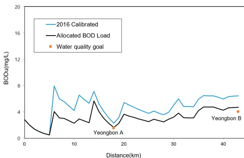
**Figure 6.** Water quality distribution in the Yeongsan River after waste load allocation (WLA) application according to the fuzzy model. The water quality goal is the target water quality for BODu in the fuzzy WLA model proposed in this study. The allocated BOD load is the water quality distribution in the Yeongsan River calculated from the fuzzy WLA model.
