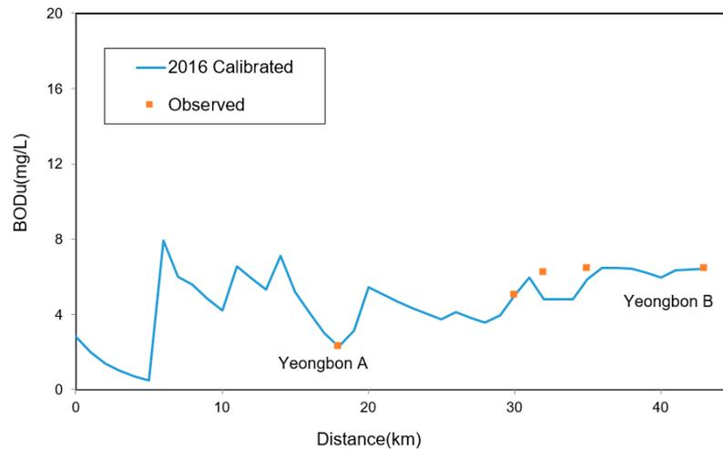
**Figure 4.** Calibration results for BOD in the main stem of the Yeongsan River: BOD<sub>u</sub> is ultimate biochemical oxygen demand, and “observed” represents the water quality measurement results for the Yeongsan River in the low-flow season in 2016. “2016 Calibrated” represents calculated BOD<sub>u</sub> after calibration in the low-flow season in 2016.
