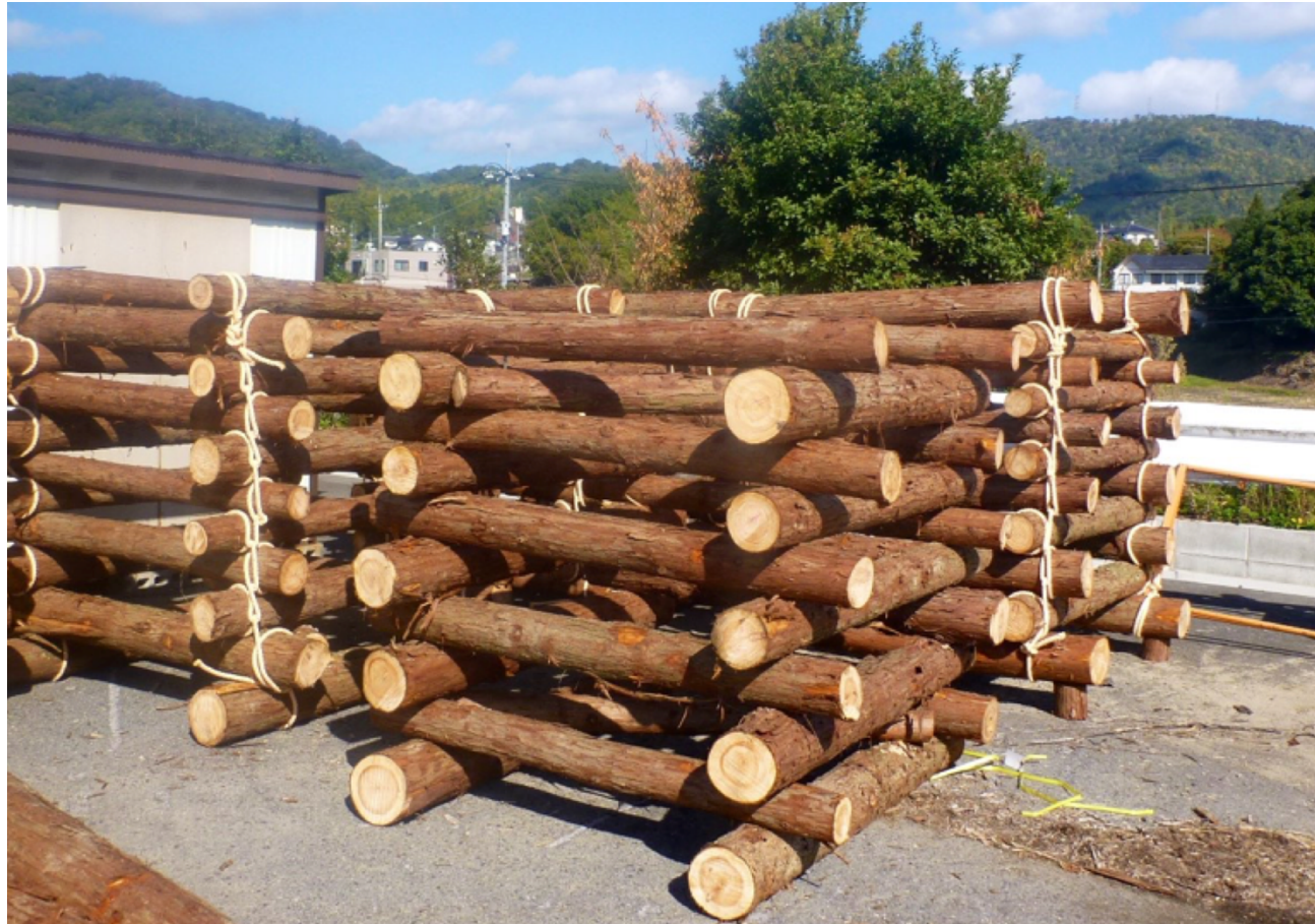
Figure S1. Photograph of ARs construction made of thinning timbers
