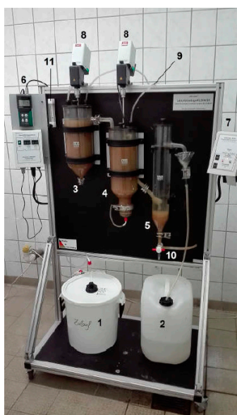
Figure 2. Lab-scale wastewater treatment systems: 1—storage tank for feed water, 2—storage tank for clarified drain water, 3—denitrification tank, 4—activation tank, 5—secondary clarification tank, 6—oxygen meter and control panel oxygen entry control, 7—control panel sludge return, 8—agitators, 9—sludge recirculation, 10—sludge recirculation, 11—volume flow measurement.
