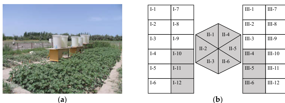
Figure 2. (a) Lysimeters where the experiment was carried out; (b) schematic diagram of the experimental site (the gray in this figure indicates the lysimeters that were not used). Note: I-1 represents the first experimental field in Field One and so on.
