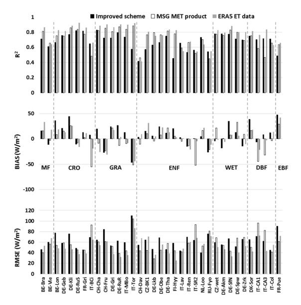
**Figure 4.** Statistical values of comparisons of instantaneous *LE* from improved scheme, MET product and ERA5 ET data with in situ measurements from FLUXNET2015 for each site (dashed lines separate sites with different land covers).
