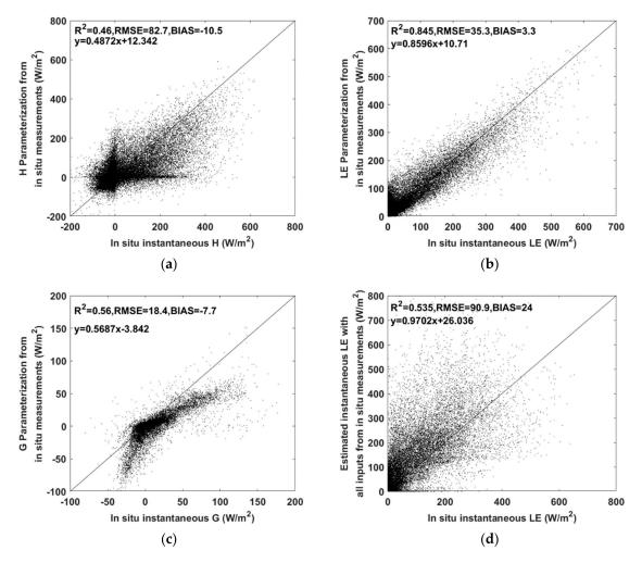
**Figure 9.** Evaluation of: (a) sensible heat flux (*H*); (b) latent heat flux (*LE*); (c) soil heat flux (*G*) parameterization by in situ measurements; and (d) estimated instantaneous *LE* with all inputs from in situ measurements.
