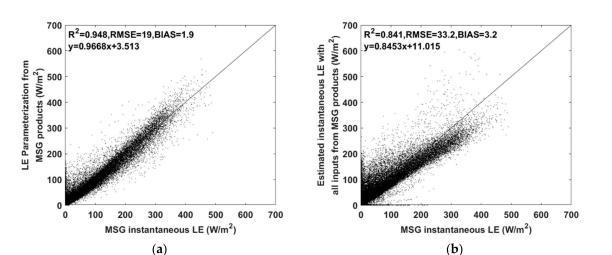
**Figure 10.** Evaluation of: (**a**) *LE* parameterization by MSG ET (MET) product; and (**b**) estimated instantaneous *LE* with all inputs from MSG products.
