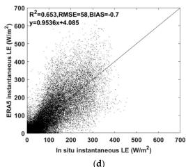
**Figure 3.** Comparisons of estimated instantaneous latent heat flux (*LE*) with in situ measurements from the FLUXNET2015 dataset: (**a**) improved method constrained by ETMonitor daily evapotranspiration (ET); (**b**) original method without constraint; (**c**) Meteosat Second Generation (MSG) ET (MET) product; (**d**) ERA5 ET data; and (**e**) their error frequency distribution histograms.
