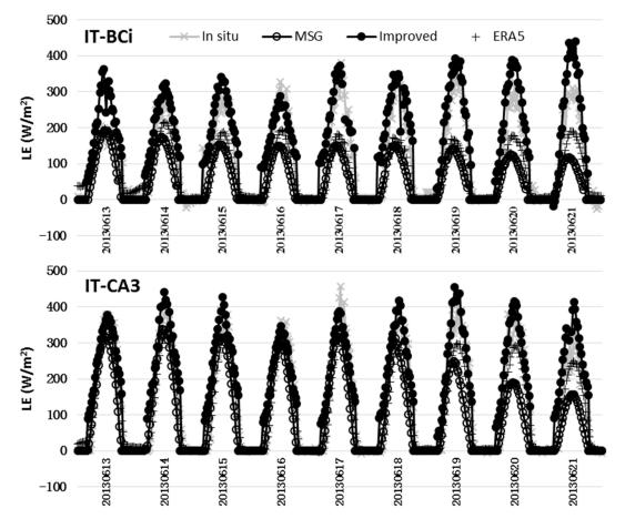
**Figure 5.** Diurnal *LE* variation from improved scheme, MET product, ERA5 ET data, and in situ measurements from FLUXNET2015 during nine consecutive days for two flux sites.
