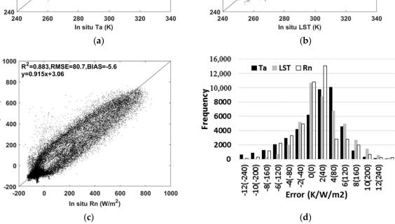
Figure 6. Comparisons of: (a) ERA5 T<sub>a</sub>; (b) MSG land surface temperature (MLST) product; and (c) MSG-calculated R<sub>n</sub> at 30 min intervals with in situ measurements from the FLUXNET2015 dataset; and (d) their error frequency histograms.
