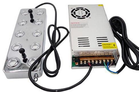
**Figure 5.** Ultrasonic water atomizer used in the experiments.
