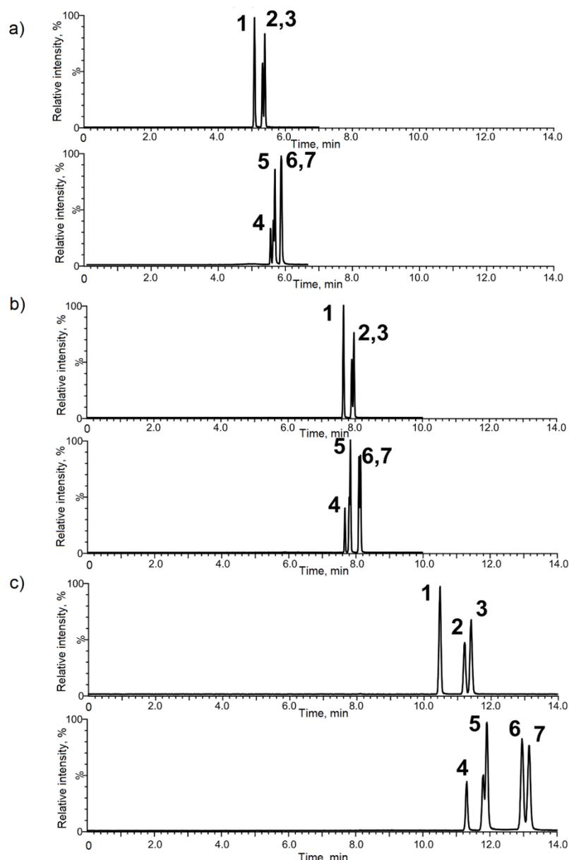
**Figure 1.** Optimization of the HPLC separation of metabolite position isomers of the toluic and methylbenzylsuccinic acids. 1 – *o*-toluic acid, 2 – *m*-toluic acid, 3 – *p*-toluic acid, 4 – 2-(1-phenylethyl)-succinic acid, 5–2-(2-methylbenzyl)succinic acid, 6–2-(3-methylbenzyl)succinic acid, and 7–2-(2-methylbenzyl)succinic acid). Acetic acid concentration in the mobile phase: (a) 0.05 %, (b) 0.1 %, and (c) 0.2 %. Column BEH C18 (50 × 2.1 mm × 1.7 μm).
