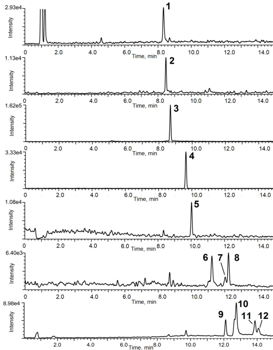
**Figure 4.** Chromatograms of a deep gas storage aquifer water sample. 1—salicylic acid, 2—phenyl-succinic acid, 3—benzoic acid, 4—4-fluorobenzoic acid C13-D' (IS), 5—benzyl-succinic acid, 6—*o*-toluic acid, 7—*m*-toluic acid, 8—*p*-toluic acid, 9—2-(1-phenylethyl)-succinic acid, 10—2-(2-methylbenzyl)-succinic acid, 11—2-(3-methylbenzyl)-succinic acid, 12—2-(4-methylbenzyl)succinic acid. Note the difference in the y-axis scales which were chosen for the maximum zoom of the chromatogram
