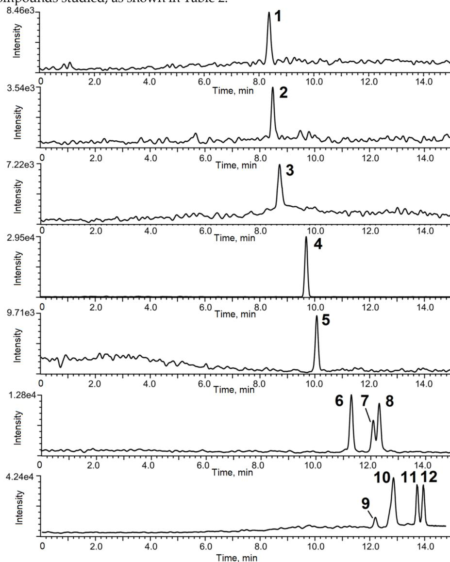
**Figure 2.** Chromatogram of metabolite standards (1 ng/mL, except for IS at 10 ng/mL). 1—salicylic acid, 2—phenylsuccinic acid, 3—benzoic acid, 4—4-fluorobenzoic acid C13-D' (IS), 5—benzylsuccinic acid, 6—*o*-toluic acid, 7—*m*-toluic acid, 8—*p*-toluic acid, 9—2-(1-phenylethyl)-succinic acid, 10—2-(2-methylbenzyl)-succinic acid, 11—2-(3-methylbenzyl)-succinic acid, and 12—2-(4-methylbenzyl)-succinic acid.
