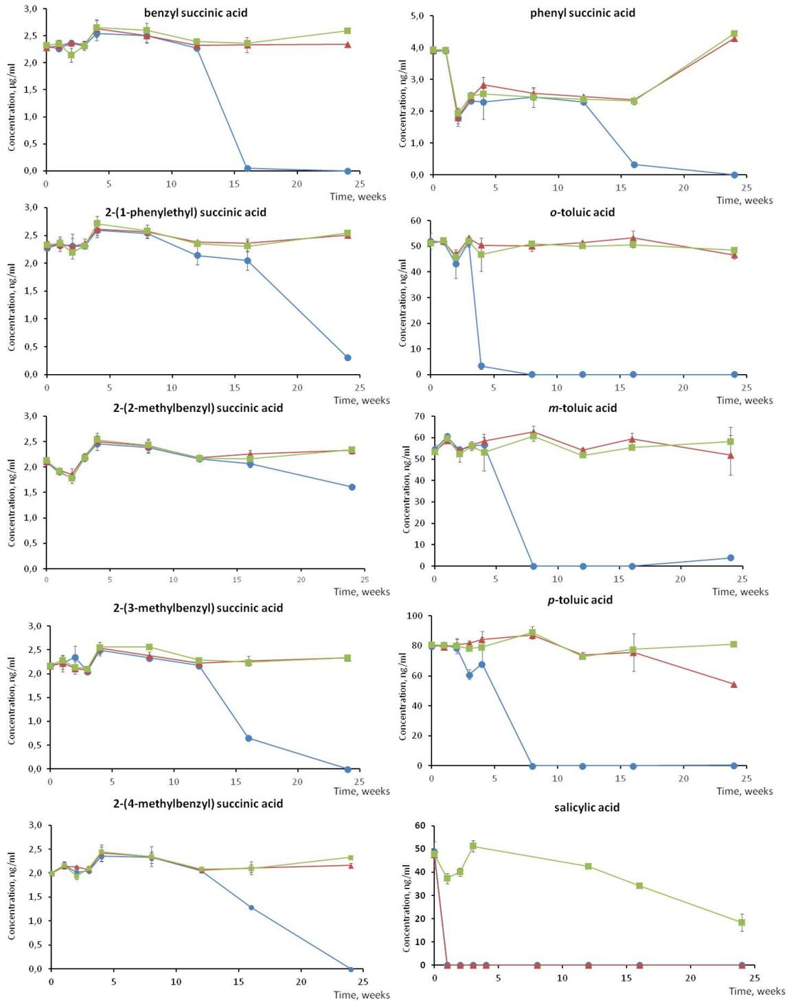
**Figure 3.** Evolution of the concentration of benzene, toluene, ethylbenzene, and andxylenes (BTEX) metabolites during sample storage at room temperature (blue curve), 4 °C (red curve) and -20 °C (green curve) over 24 weeks (deep gas storage aquifer water spiked with known initial concentration for the purpose of a stability study).
