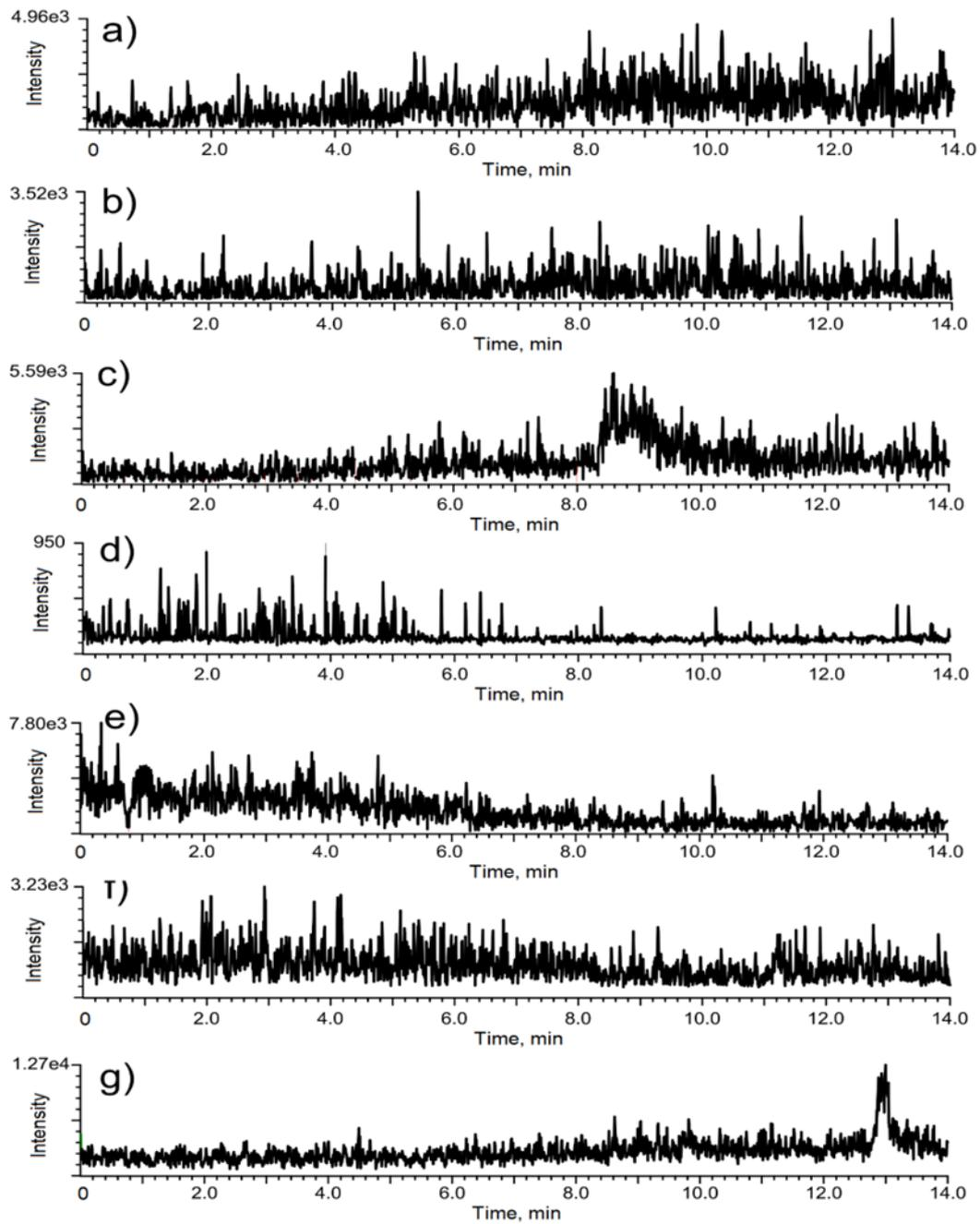
**Figure 5.** Chromatograms of a blank corresponding to the deep gas storage aquifer water sample (cf. Figure 4. measured for m/z (a) 135.9 → 93.0, (b) 193.0 → 149.0, (c) 120.9 → 77.0, (d) 144.0 → 99.1, (e) 207.0 → 163.1, (f) 135.0 → 91.0, (g) 221.1 → 177.1.
