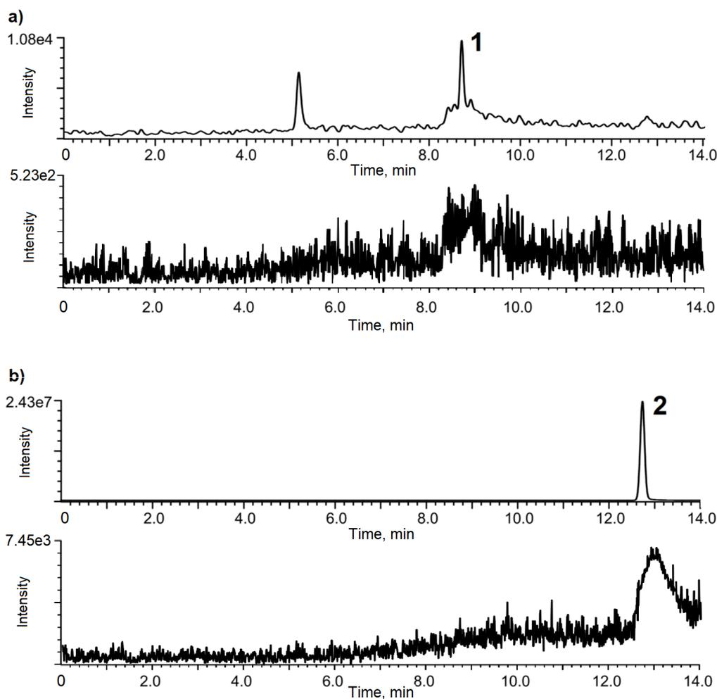
**Figure 6.** Chromatogram of biological culture sample: (a) benzoic acid (1) (b) 2-(2-methylbenzyl)-succinic acid (2); sample and blank chromatograms are shown on upper and lower panels, respectively. Note the difference in the y-axis scales which were chosen for the maximum zoom of the chromatogram.
