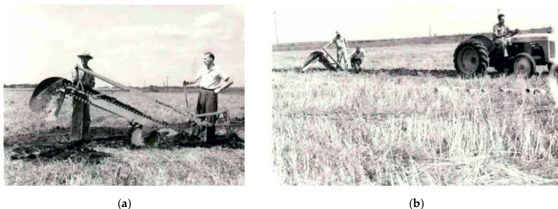
Figure 20. (a) Aashmar's Draining Plow (b) In use [77].
