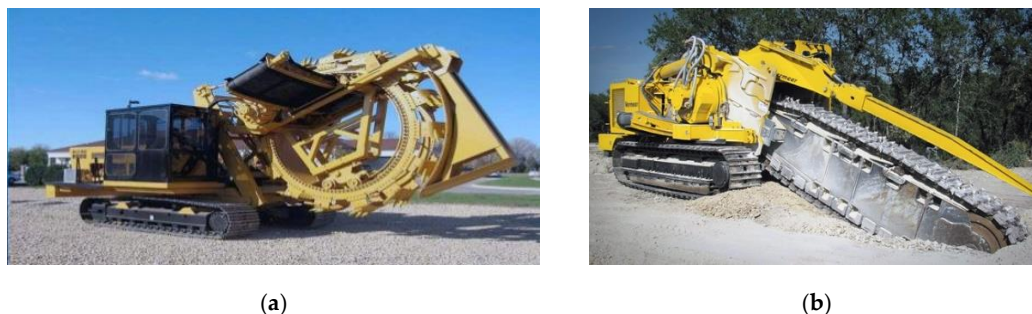
Figure 21. Trencher machines: (a) wheel type [82]; (b) ladder or chain type [83].
