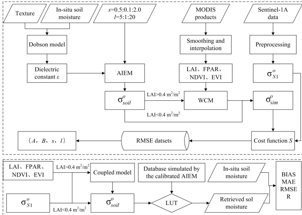
**Figure 4.** Flowchart for the model calibration and the soil moisture retrieval. The AIEM and WCM stand for the advanced integral equation model and the water cloud model, respectively. The LUT is the look-up-table. The BIAS (the mean bias), MAE (mean absolute error), RMSE (root mean square error),  $R$  (Pearson correlation coefficient) are statistical indicators.
