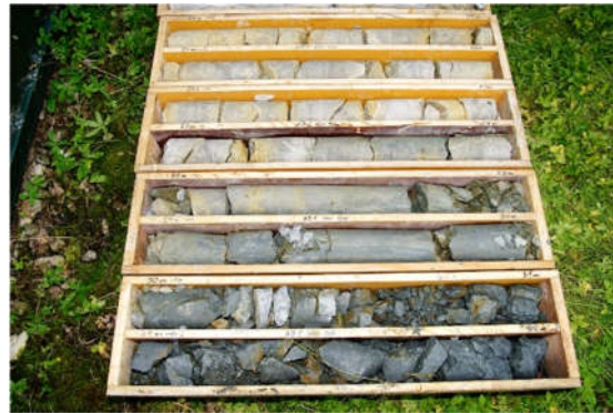
Figure 7. Rock samples of depth from 24 m to 31 m in well N.
