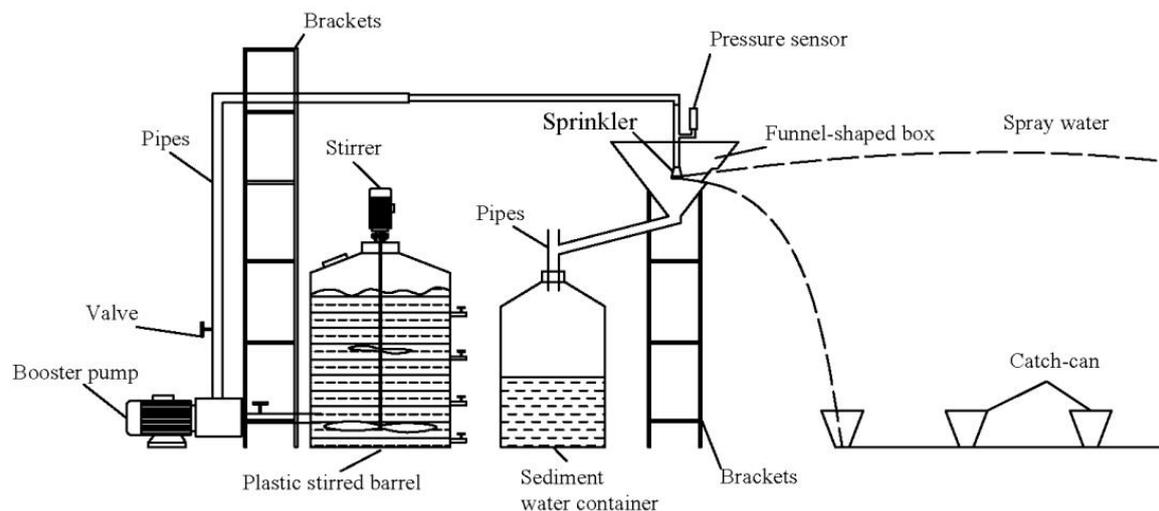
**Figure 1.** Experimental setup for sprinkler sediment-water distribution.
