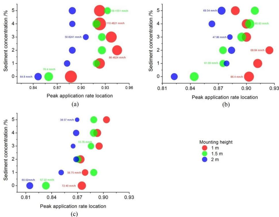
Figure 5. Migration of peak application rate with different sediment concentrations. Note: (a) 100 kPa, (b) 150 kPa, (c) 200 kPa.
