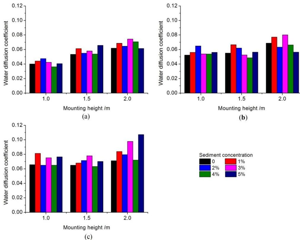
**Figure 6.** Spray water diffusion coefficient with various sediment contents at different working heights. Note: (a) 100 kPa, (b) 150 kPa, (c) 200 kPa.
