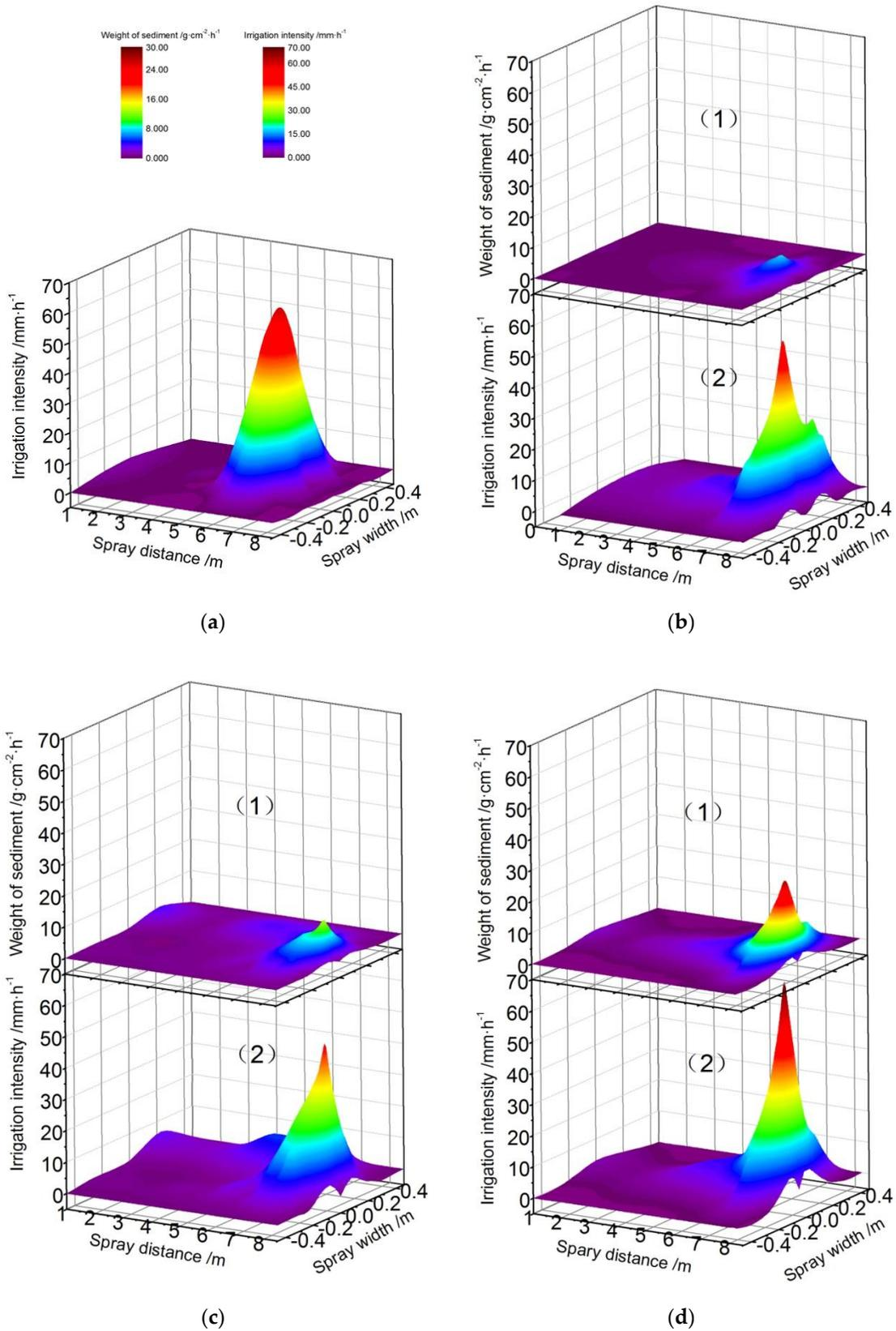
**Figure 3.** Water and sediment distribution patterns of one groove with 2 m mounting height at 150 kPa. Note: (a) clean water; (b) 1% sediment concentration; (c) 3% sediment concentration; (d) 5% sediment concentration.
