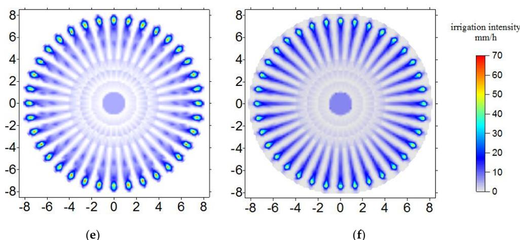
**Figure 4.** The effect of sediment contents on water distribution pattern with 1.5 m mounting height at 150 kPa. Note: (a) clean water, (b) 1% sediment content, (c) 2% sediment content, (d) 3% sediment content, (e) 4% sediment content, (f) 5% sediment content.
