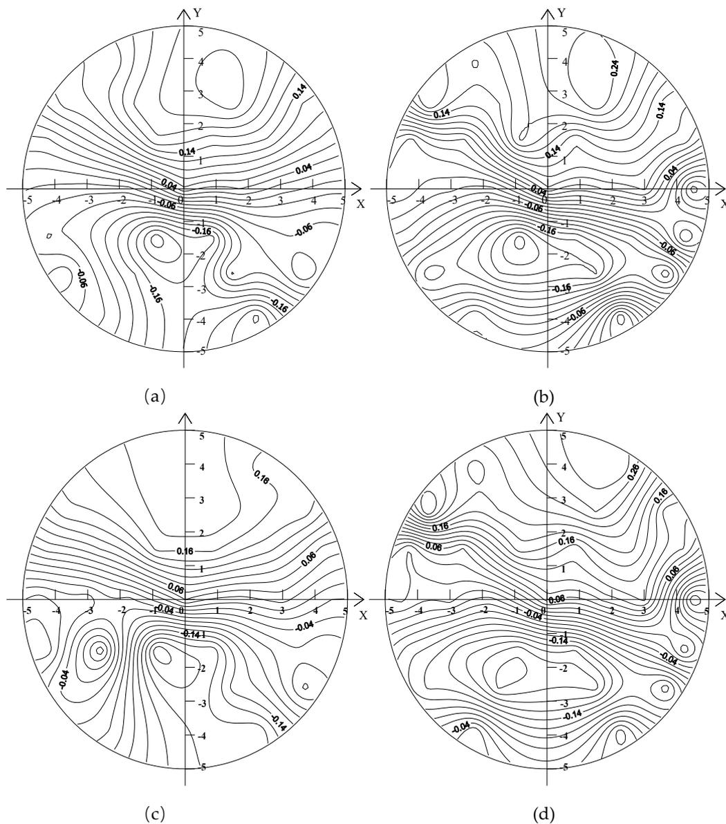
**Figure 6.** Circumferential velocity distributions of the upstream sections of capsules: (a)  $L/d = 2.5$ ,  $Z = 3$  m; (b)  $L/d = 2.14$ ,  $Z = 3$  m; (c)  $L/d = 2.5$ ,  $Z = 0.1$  m; and (d)  $L/d = 2.14$ ,  $Z = 0.1$  m.
