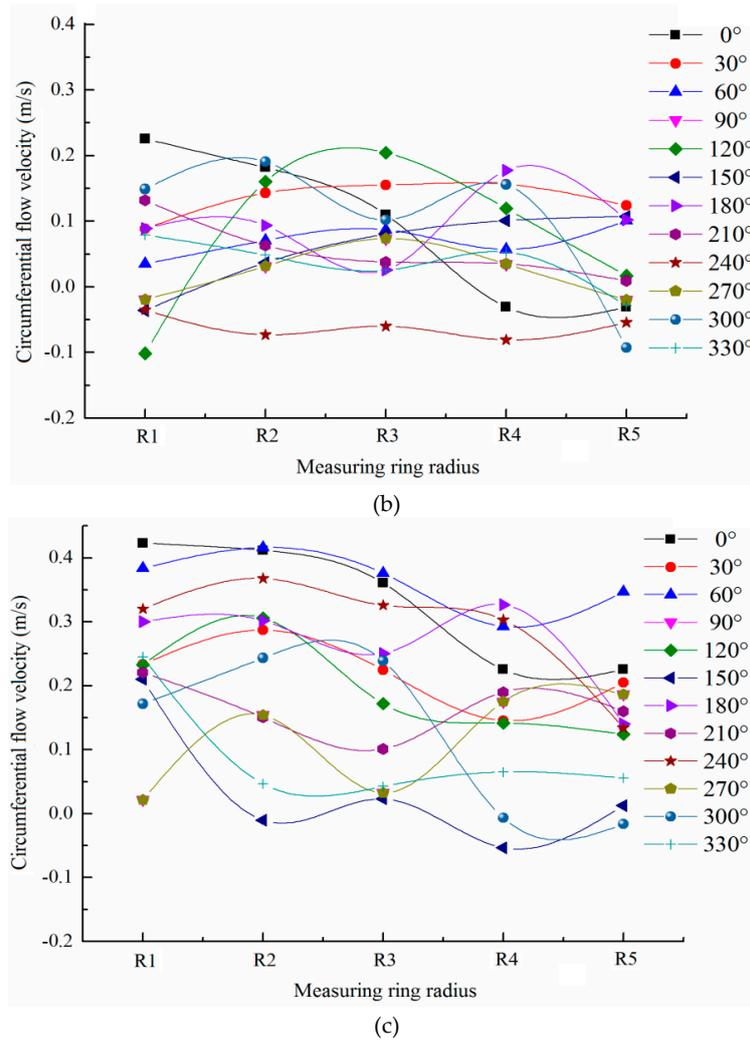
**Figure 15.** Circumferential velocity of the same polar axis: (a) rear section; (b) middle section; and (c) front section.
