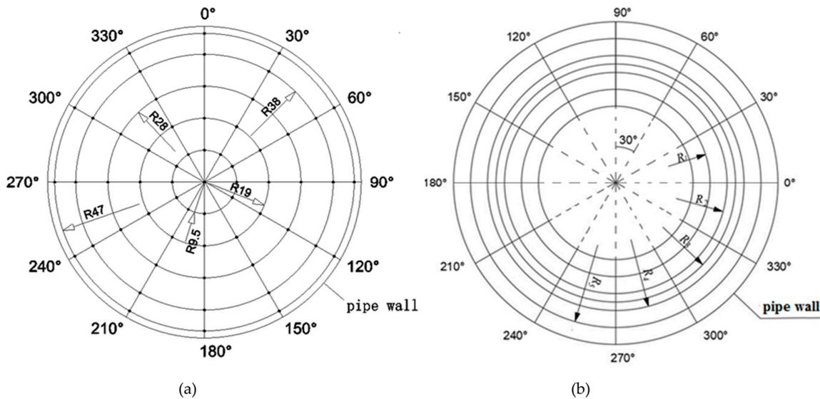
**Figure 3.** Layout of measuring points of sections: (a) the front and rear sections of capsule and (b) the annular gap section.
