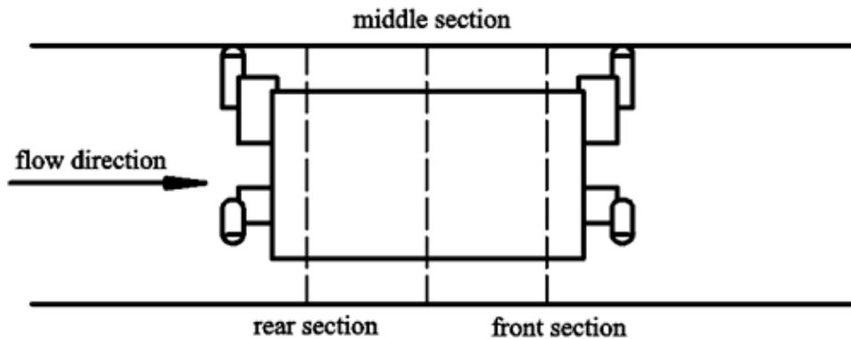
**Figure 4.** Schematic diagram of annular gap section division of capsule.
