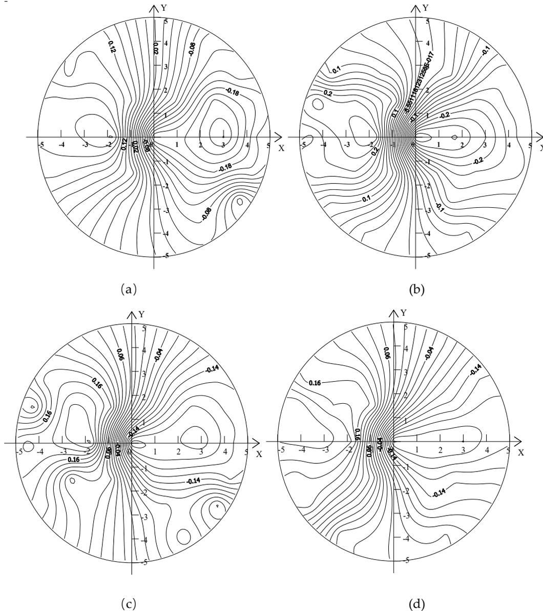
**Figure 10.** Radial velocity distribution of the downstream sections of capsules: (a)  $L/d = 2.5$ ,  $Z = 0.2$  m; (b)  $L/d = 2.14$ ,  $Z = 0.2$  m; (c)  $L/d = 2.5$ ,  $Z = 3$  m; and (d)  $L/d = 2.14$ ,  $Z = 3$  m.
