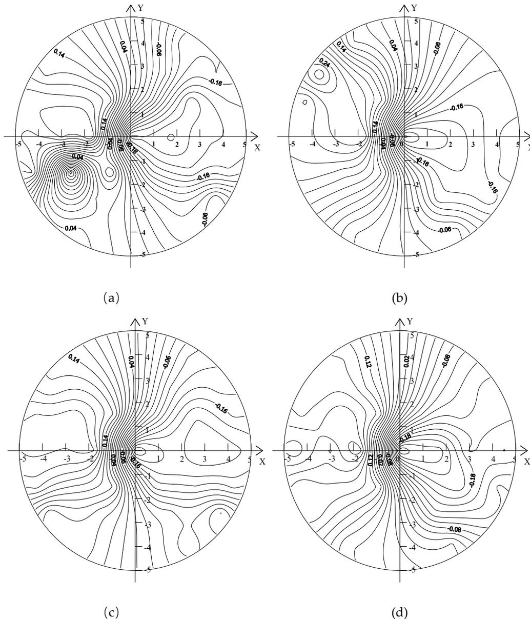
**Figure 7.** Radial velocity distributions of the upstream sections of capsules: (a)  $L/d = 2.5$ ,  $Z = 3$  m; (b)  $L/d = 2.14$ ,  $Z = 3$  m; (c)  $L/d = 2.5$ ,  $Z = 0.1$  m; and (d)  $L/d = 2.14$ ,  $Z = 0.1$  m.
