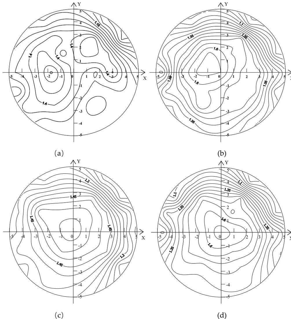
**Figure 8.** Axial velocity distributions of the downstream sections of capsules: (a)  $L/d = 2.5$ ,  $Z = 0.2$  m; (b)  $L/d = 2.14$ ,  $Z = 0.2$  m; (c)  $L/d = 2.5$ ,  $Z = 3$  m; and (d)  $L/d = 2.14$ ,  $Z = 3$  m.
