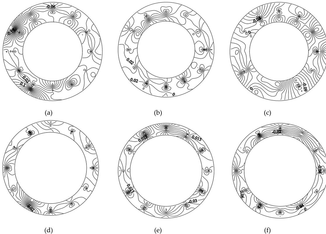
**Figure 17.** Radial flow velocity distribution of annular gap sections of the capsules: (a)  $L/d = 2.5$ , rear section; (b)  $L/d = 2.5$ , middle section; (c)  $L/d = 2.5$ , front section; (d)  $L/d = 2.14$ , rear section; (e)  $L/d = 2.14$ , middle section; and (f)  $L/d = 2.14$ , front section.
