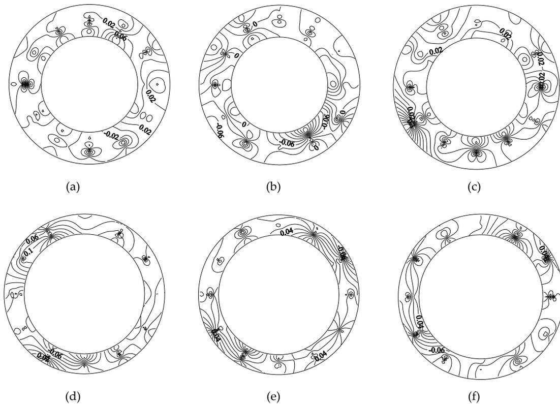
**Figure 14.** Circumferential flow velocity distribution of annular gap sections of the capsules: (a)  $L/d = 2.5$ , rear section; (b)  $L/d = 2.5$ , middle section; (c)  $L/d = 2.5$ , front section; (d)  $L/d = 2.14$ , rear section; (e)  $L/d = 2.14$ , middle section; and (f)  $L/d = 2.14$ , front section.
