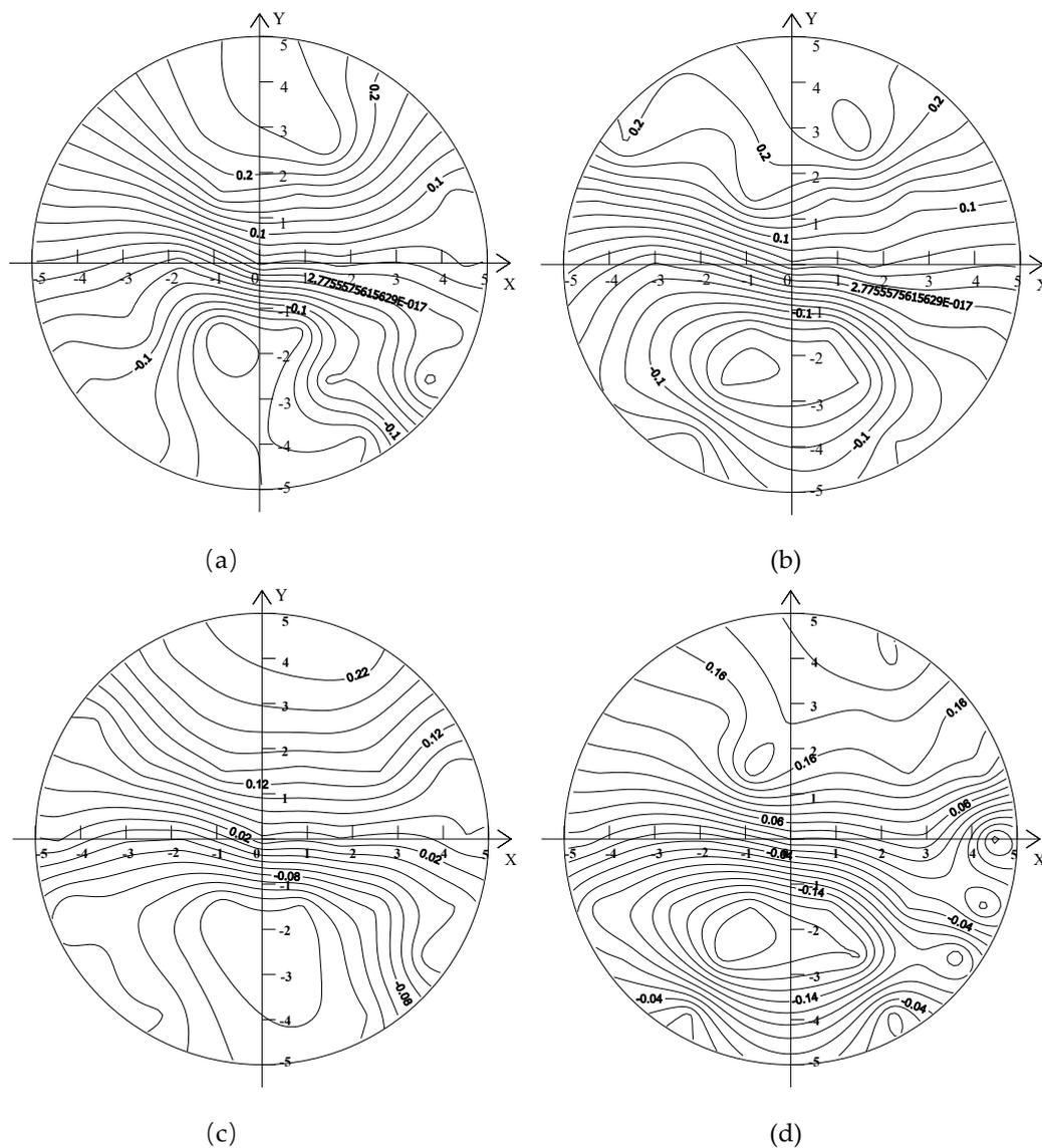
**Figure 9.** Circumferential velocity distribution of the downstream sections of capsules: (a)  $L/d = 2.5$ ,  $Z = 0.2$  m; (b)  $L/d = 2.14$ ,  $Z = 0.2$  m; (c)  $L/d = 2.5$ ,  $Z = 3$  m; and (d)  $L/d = 2.14$ ,  $Z = 3$  m.
