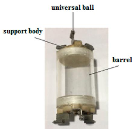
Figure 1. Structural diagram of wheeled capsule.
