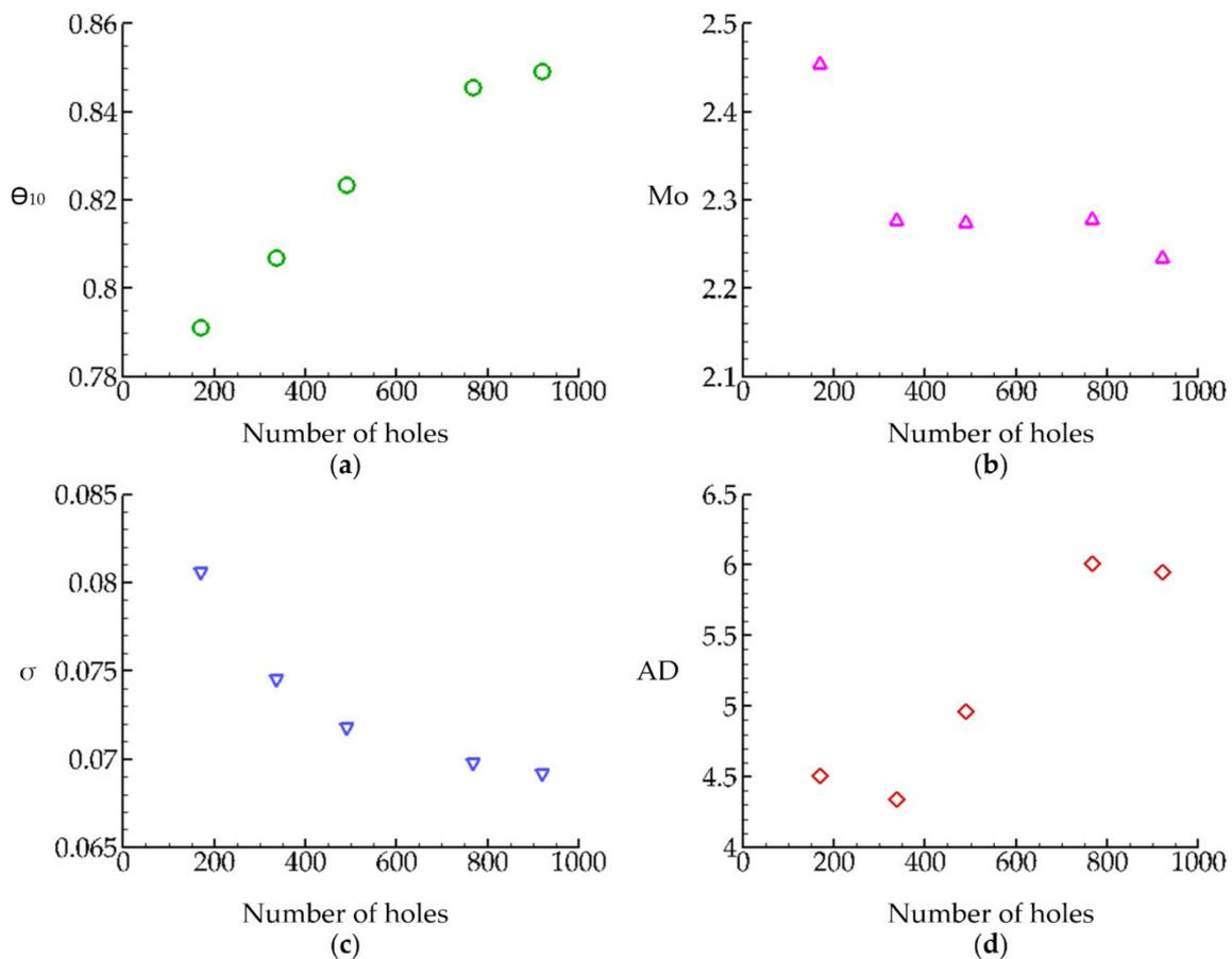
**Figure 9.** Variation of efficiency indexes with the number of holes for the constant solidity ratios of 95% in Section 1, 80% in Section 2 and 65% in Section 3: (a) baffling factor, (b) Mo index, (c) dispersion index and (d) AD index.
