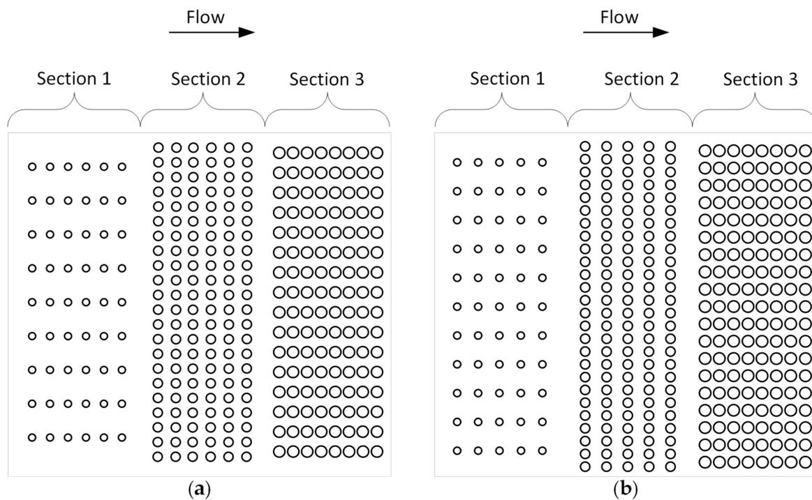
**Figure 5.** Sketch of the manufactured baffles showing the hole distribution on the baffle: solidity ratio decreases in the flow direction (a) Design 2; (b) Design 7.
