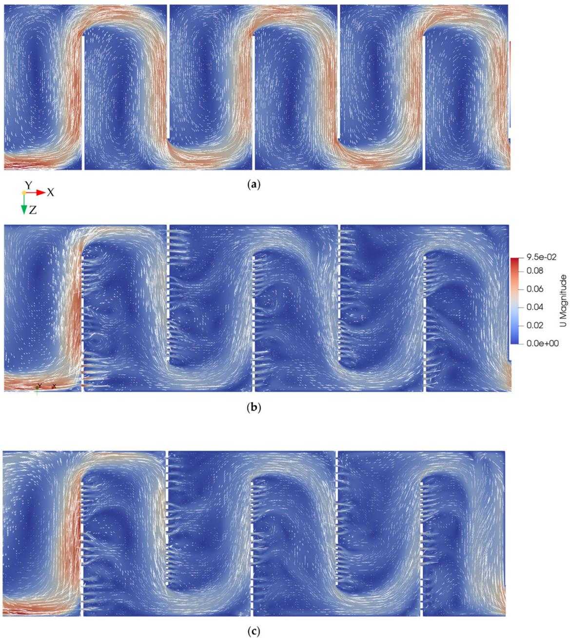
**Figure 7.** Velocity vectors on a horizontal plane located at the mid-depth of the tank: (a) conventional design; (b) Design 2; (c) Design 7.
