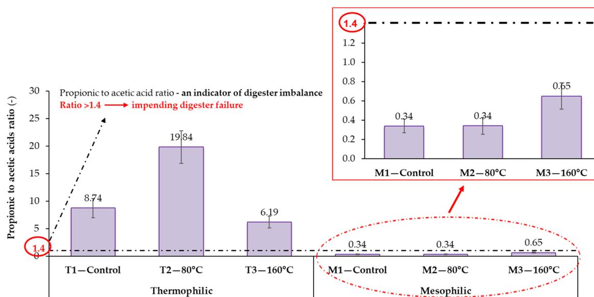
**Figure 3.** Ratios of propionic to acetic acids in the thermophilic and mesophilic digesters.
