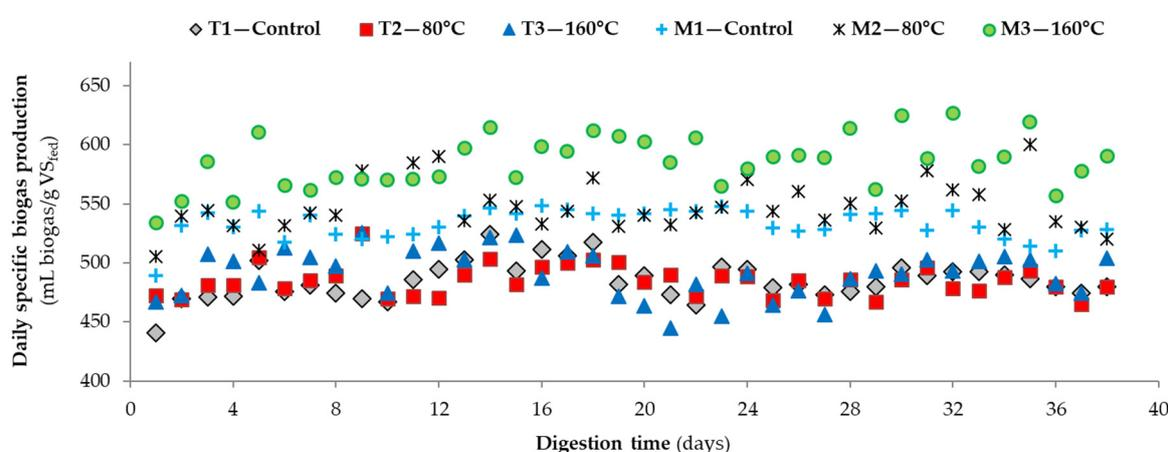
**Figure 1.** Evolution of specific biogas yields of thermophilic and mesophilic digesters during the operating period after reaching a steady state (0 °C and 1 atm).
