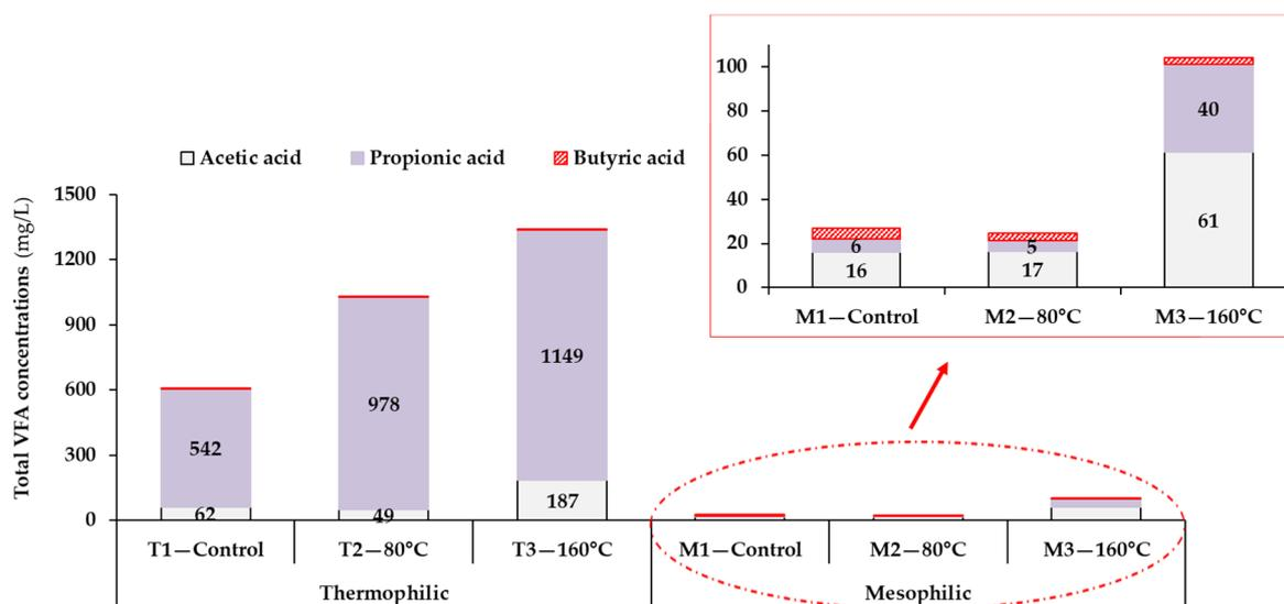
**Figure 2.** Concentrations of acetic, butyric, and propionic acids in the thermophilic and mesophilic digesters operated under high organic loading rates.
