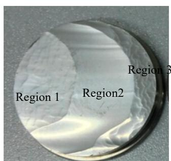
**Figure 19.** Wear of test sample at 316 mm.
