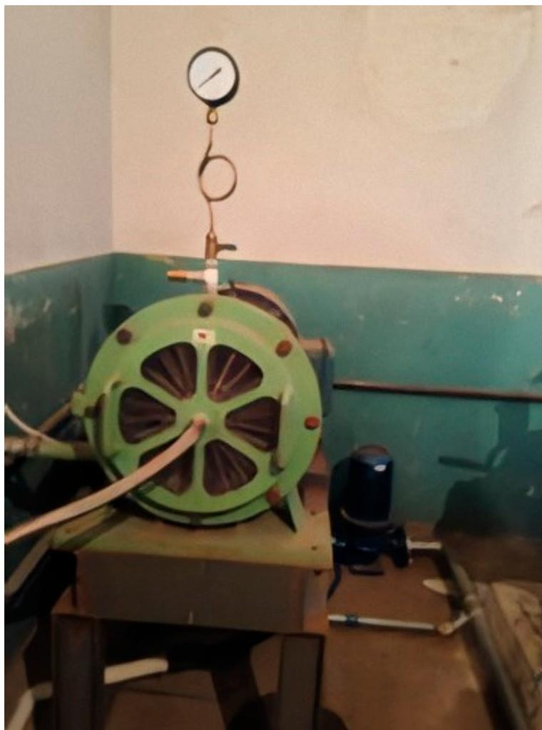
**Figure 2.** Rotating disc test rig.
