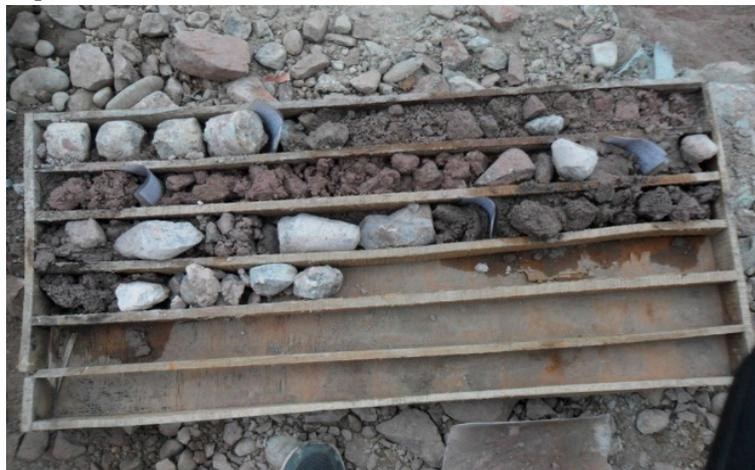
**Figure 4.** Photo of the rock core sample.
