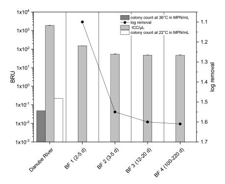
**Figure 5.** ICC monitored in various RBF wells in Budapest and their travel times in days, BF 1 = Csepel water plant, well No. 1, BF 2 = Tahi 1, well No. 5, BF 3 = Tahi 2 well No. 5, BF 4 = Szigetujfalu, well No. 7 with error bars rep-resenting standard deviation for those points, FCM samples were stained with SYBER®Green and propidiumiodide, HPC data were provided by Budapest Water Works Ltd. Modelled travel times may overlap depending on Danube River water levels.
