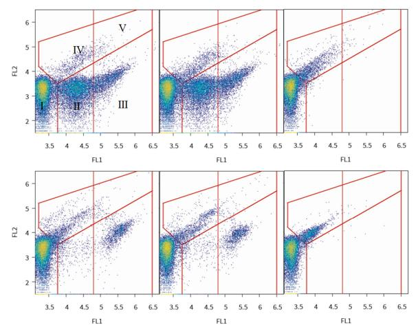
**Figure 4.** Dot-plots of water treatment trains in CI, Line 1: RBF, aeration, ozonation; Line 2: sandfilter, ultraviolet (UV-C) disinfection, assignments of Sections I to III: Background Signal, Intact LNAC, Intact HNAC, Sections IV-V: Lysed Cells, x-axis: Flourescence Signal 1 (FL1), y-axis: Flourescence Signal 2 (FL2).
