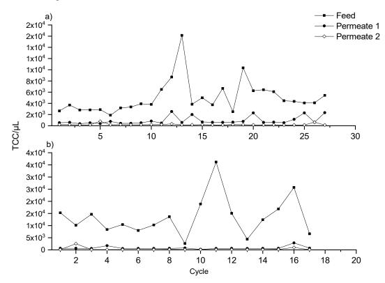
**Figure 7.** Continuous determination of total cell count (TCC) in Elbe River water (feed), Permeate 1 and Permeate 2, (**a**) 26 April–29 May 2019, (**b**) 2 May–4 May 2019, samples were stained with SYBER®Green and propidiumiodide.
