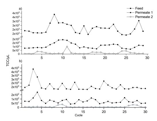
**Figure 6.** Continuous determination of total cell count (TCC) in flocculated Elbe River water (feed), Permeate 1 and Permeate 2, (**a**) 9–12 November 2018, (**b**) 19–22 November 2018), samples were stained with SYBER® Green.
