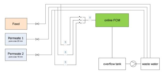
Figure 1. Scheme of online flow-cytometry (FCM) sampling system.
