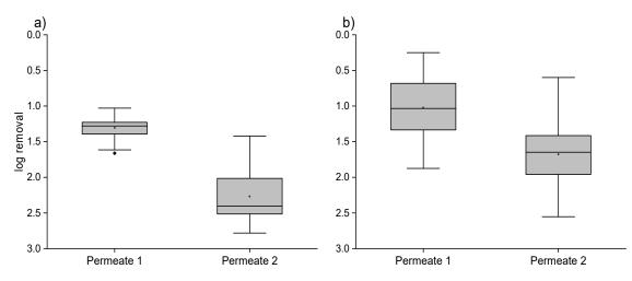
**Figure 8.** Differences in log removal rates of Permeate 1 and Permeate 2 in (**a**) flocculated Elbe river water *t*-test, n = 59, p < 0.05, n = 59 and (**b**) Elbe River water, t-test, n = 44, p < 0.05.
