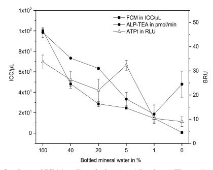
**Figure 2.** Correlation of FCM (n = 5), total adenosine triphosphate (ATPt, n = 3) and alkaline phosphatase-total enzymatic activity (ALP-TEA, n = 3) for measuring total biomass related units (BRU), samples from bottled mineral water (Evian) were diluted with ultrapure water from the same bottle, based on a method described in [13]. FCM samples were stained with SYBER®Green and propidiumiodide, error bars indicate standard deviation on samples.
