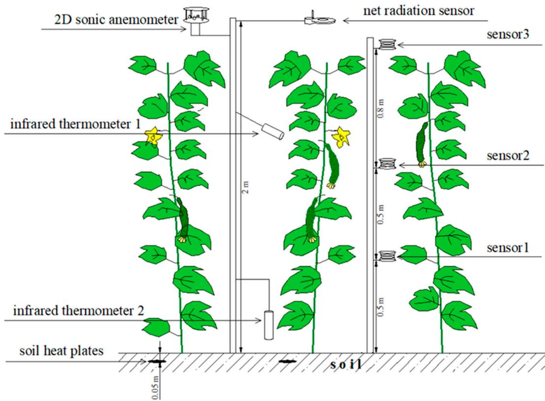
Figure 1. A schematic view of the sensor locations.
