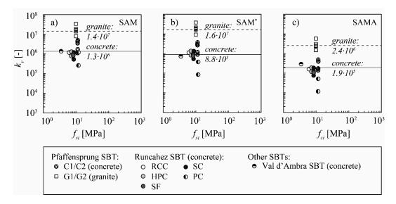
**Figure 14.** Abrasion coefficient  $k_v$  as a function of splitting tensile strength of various SBT invert materials for (**a**) SAM, (**b**) SAM<sup>\*</sup> and (**c**) SAMA.
