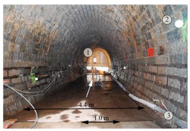
**Figure 2.** Measurement installation in Pfaffensprung SBT at test field location 1 during scanning in March 2014, (1) terrestrial laser scanner (TLS), (2) temporary mounted targets and (3) ground water drainage, view in flow direction from high-strength concrete (C1) over granite pavement (G1) to SBT outlet.
