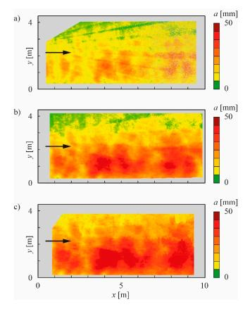
**Figure 5.** High-resolution abrasion maps of the 10 m long high-strength concrete test field C1 installed at test location 1 in Pfaffensprung SBT after (**a**) one, (**b**) two and (**c**) four operational years (the grey colored areas could not be scanned due to ground water drainage installation).
