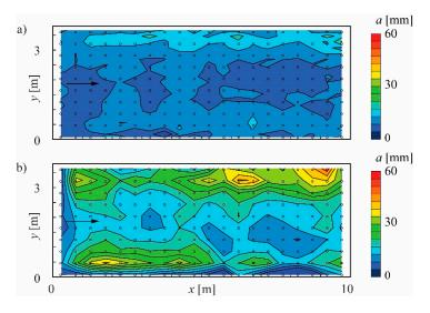
**Figure 11.** Abrasion depths of the silica fume concrete (SC) test field in Runcahez SBT in (**a**) 1999 after four years of operation and (**b**) 2014 after 19 years of operation (circles represent measurement points).
