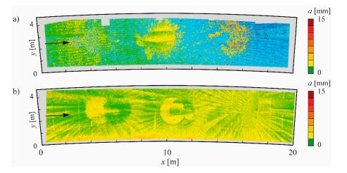
**Figure 8.** High-resolution abrasion maps of the 20 m long granite test filed G2 installed at test location 2 in Pfaffensprung SBT after (**a**) one and (**b**) two operational years (blue colored points mark theoretically negative abrasion depths corresponding to detection uncertainty; grey areas could not be scanned due to ground water drainage installation).
