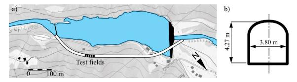
**Figure 3.** (a) Overview and (b) cross section of the Runcahez SBT (position 46°40′45.0″ N 8°58′05.7″ E; adapted from [18]).
