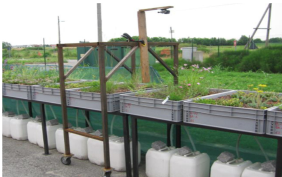
Figure 5. The mobile stand with a camera to take photos of the plant cover.
