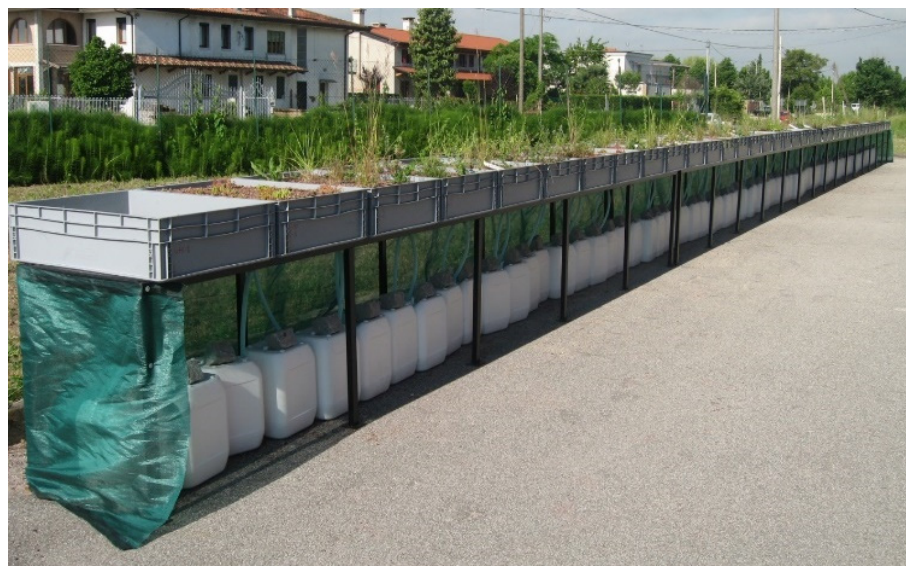
Figure 2. The microcosms of green roofs at the experimental site of Agripolis Campus.
