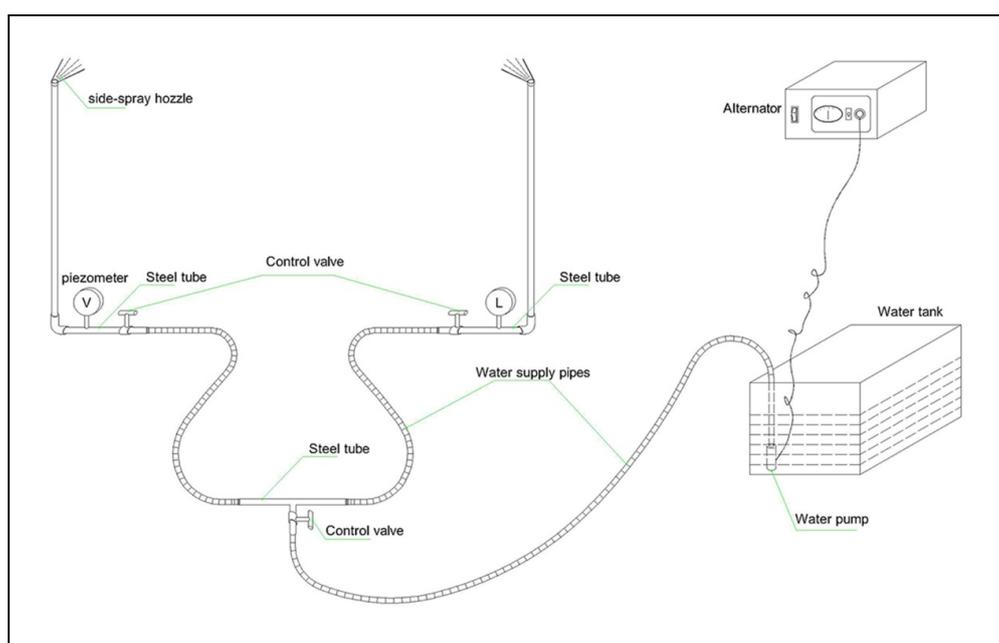
**Figure 3.** Schematic of the side-spray rainfall simulation system used in the present study.
