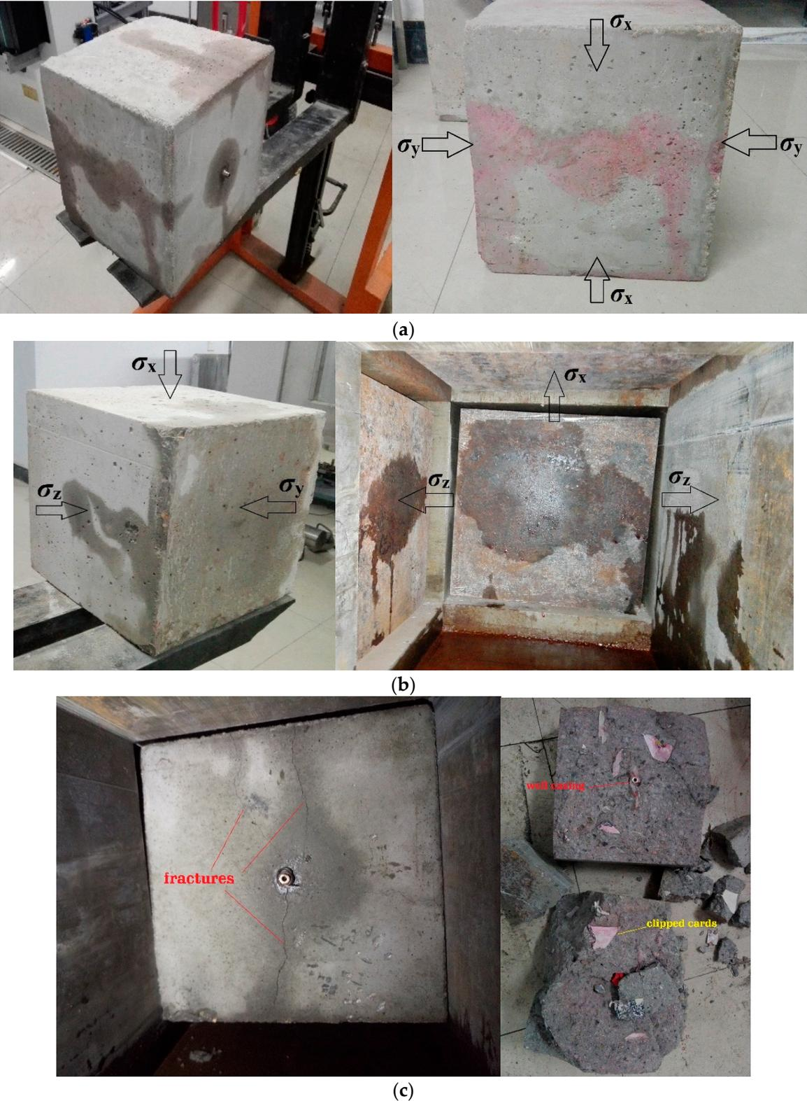
Figure 10. Fracture morphology of H1 (a), H2 (b), and F1 (c).
