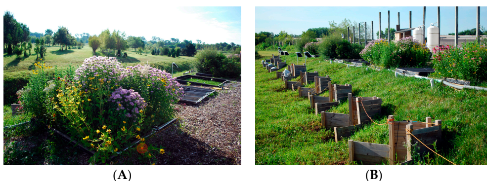
Figure 2. Twelve closed-hydrology mesocosms were established along a berm to monitor drainage responses to inputs of stormwater. Four vegetative treatments were used: turfgrass, prairie plants, shrubs, and controls lacking vegetation (A). Each mesocosm drained freely to a flow monitoring station located behind a wooden retaining wall (B).
