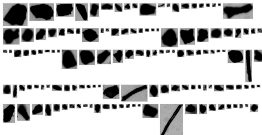
**Figure 2.** Microscopic images of some road-deposited sediment (RDS) particles of the sample ECL, captured using dynamic image analysis. The particle shape of the other samples was comparable. The images are not scaled.
