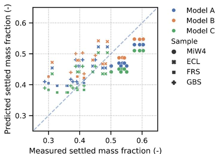
**Figure 5.** Comparison between measured and predicted settled mass fraction by Models A, B, and C of all samples (MiW4, ECL, FRS, and GBS);  $n = 33$ .
