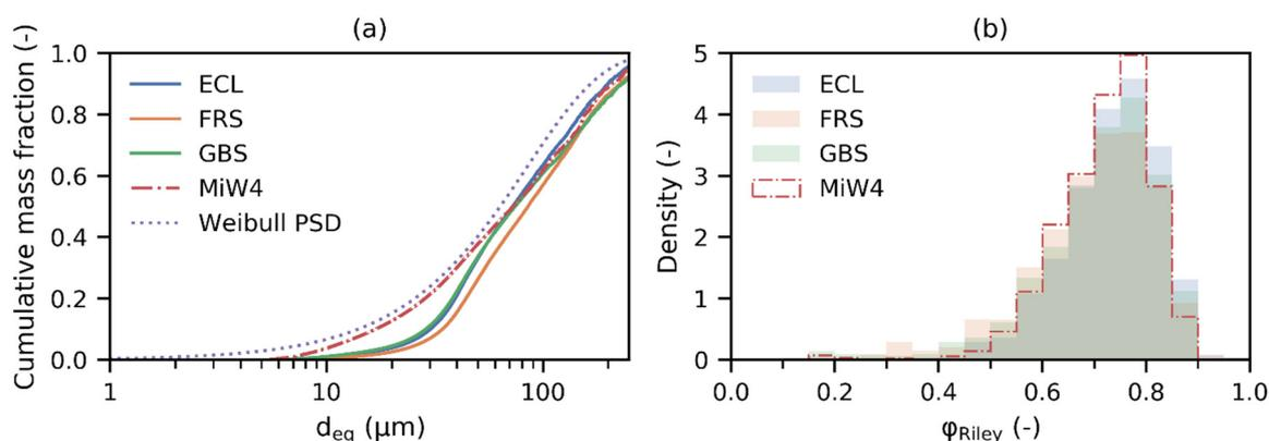
**Figure 1.** (a) Particle size distribution (PSD) of the analyzed samples and the fitted Weibull PSD used for the subsequent modeling, particle count: Eckenheimer Landstraße (ECL)  $n = 515,545$ ; Frauensteinstraße (FRS)  $n = 593,302$ ; Glauburgstraße (GBS)  $n = 540,036$ ; MiW4  $n = 501,254$ . (b) Mass fraction weighted histogram of  $\phi_{Riley}$  of the analyzed samples, particle count: ECL  $n = 130,986$ ; FRS  $n = 211,209$ ; GBS  $n = 134,392$ ; MiW4  $n = 57,973$ .
