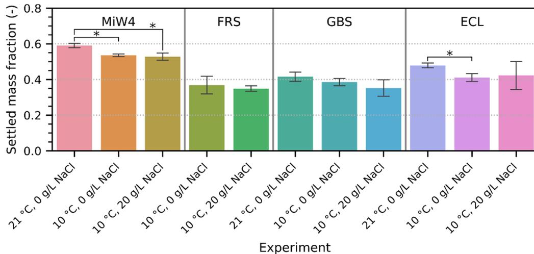
**Figure 3.** Settled mass fraction in the settling experiments with varying temperatures (21 and 10 °C) and NaCl concentrations (0 and 20 g/L);  $n = 3$  for each experiment. The error bars indicate the standard deviation; the asterisks (\*) indicate statistically significant differences between two experiments ( $p < 0.05$ ). Experiment FRS 21 °C 0 g/L NaCl was not conducted due to low sample quantity.
