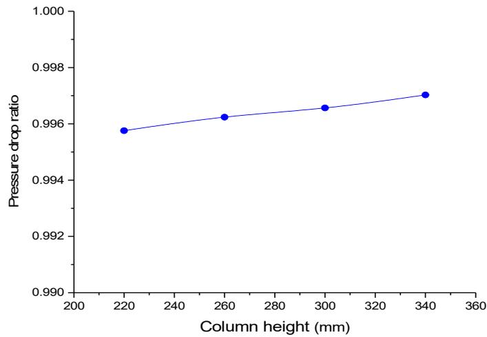
Figure 12. Effect of column height on the pressure drop ratio.
