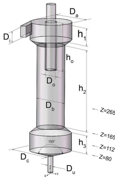
**Figure 3.** Structural diagram of the hydrocyclone.
