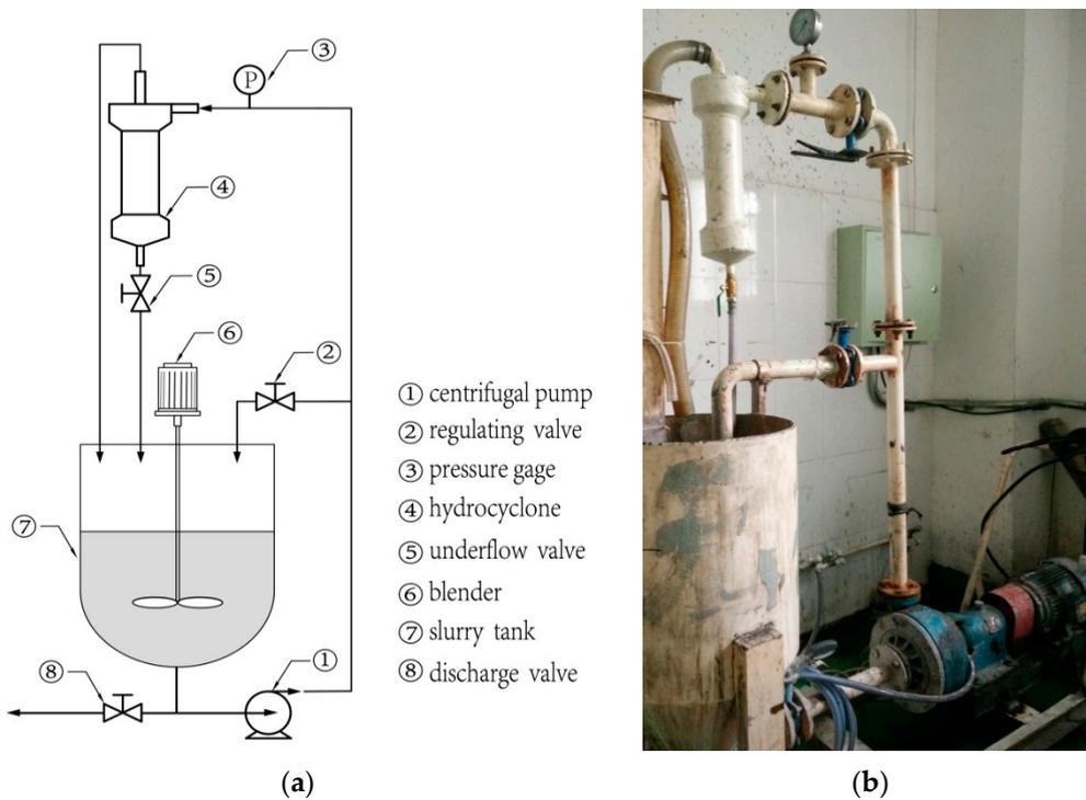
Figure 5. Schematic diagram of the (a) experimental system and (b) experimental device.
