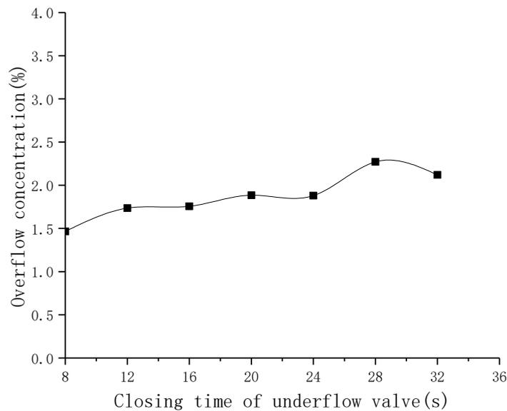
**Figure 18.** Effect of closing time of the underflow valve on overflow concentration.
