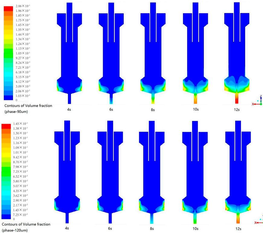
Figure 16. Cloud diagram of the volume fraction change for particles.
