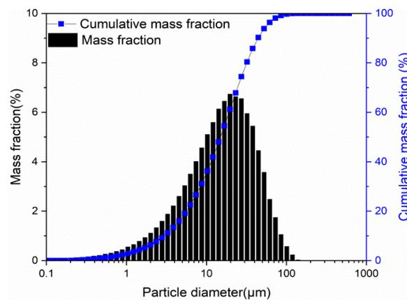
Figure 6. Particle size distribution in the experiment.
