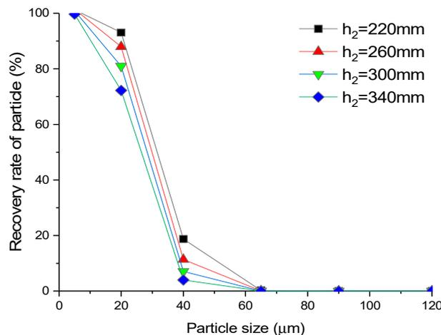
**Figure 11.** Effect of column height on the recovery rate of overflow particles.
