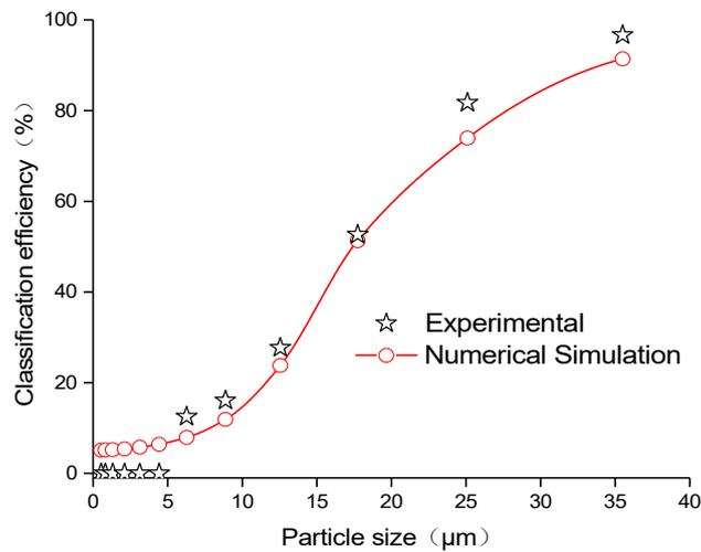
**Figure 2.** Comparison of classification efficiency curves between numerical simulation and experiment.
