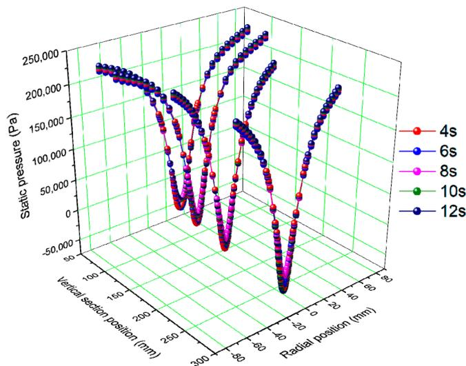
Figure 13. Distribution curve of static pressure.
