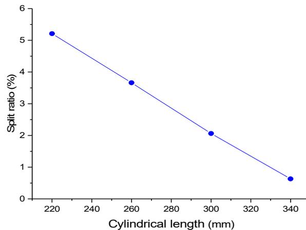
**Figure 10.** Effect of column height on the split ratio.
