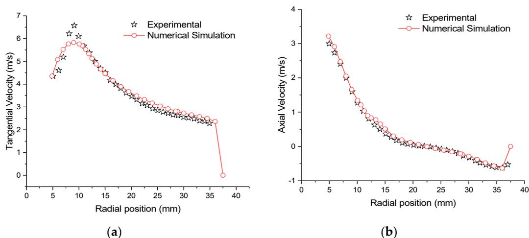
**Figure 1.** Comparison of distribution of tangential velocity (a) and axial velocity (b).
