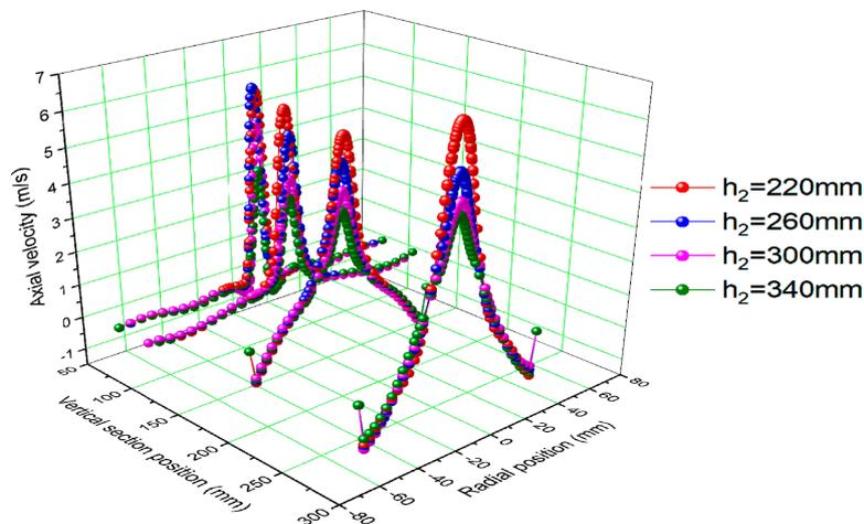
Figure 9. Distribution curve of axial velocity.
