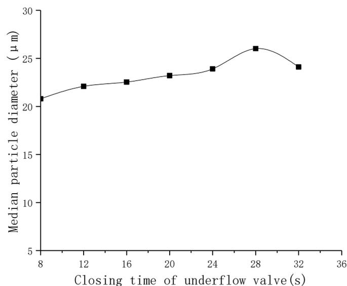
**Figure 19.** Effect of closing time of the underflow valve on median diameter of overflow particles.
