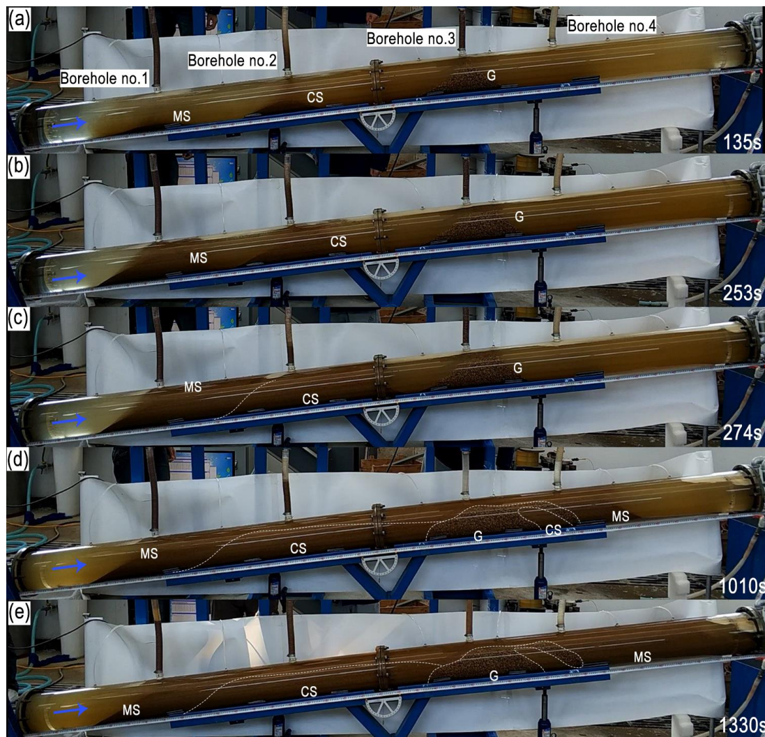
Figure 5. Aggregate deposits in Trial No. 2, with the order of pouring fine particles upstream and coarse particles downstream. (a) at 135 s, (b) at 253 s, (c) at 274 s, (d) at 1010 s, (e) at 1330 s.
