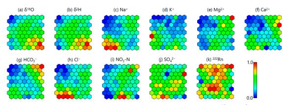
**Figure 10.** Component planes of the isotopic and hydrochemical parameters: (a)  $\delta^{18}$ O, (b)  $\delta^{2}$ H, (c) Na<sup>+</sup>, (d) K<sup>+</sup>, (e) Mg<sup>2+</sup>, (f) Ca<sup>2+</sup>, (g) HCO<sub>3</sub><sup>-</sup>, (h) Cl<sup>-</sup>, (i) NO<sub>3</sub>-N, (j) SO<sub>4</sub><sup>2-</sup>, and (k) <sup>222</sup>Rn. Each plane shows the standardized value of each parameter (transformed to the range from 0 to 1) in each node.
