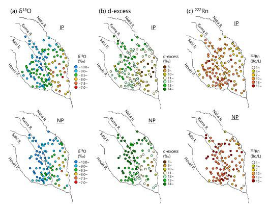
**Figure 9.** Distributions of (**a**)  $\delta^{18}$ O, (**b**) d-excess, and (**c**) the <sup>222</sup>Rn concentration in groundwater in the IP (upper maps) and NP (lower maps).
