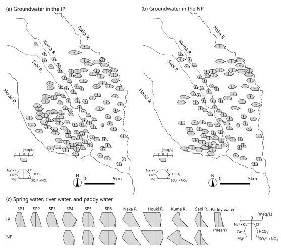
Figure 5. Hexa-diagrams of groundwater, spring water, river water, and paddy water.
