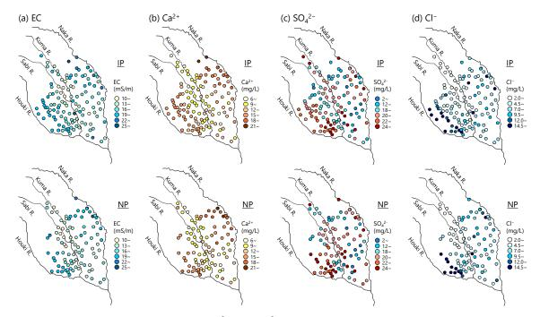
**Figure 7.** Distributions of (**a**) EC, (**b**)  $Ca^{2+}$ , (**c**)  $SO_4^{2-}$ , and (**d**)  $Cl^-$  concentrations in the groundwater. The upper and lower maps show the data in the IP and NP, respectively.
