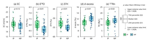
**Figure 16.** Comparison of groundwater EC values and isotopic compositions between the IP and NP at observation sites classified into group 2 in the IP.
