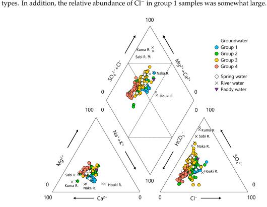
Figure 13. Trilinear diagram of the four groundwater groups.
