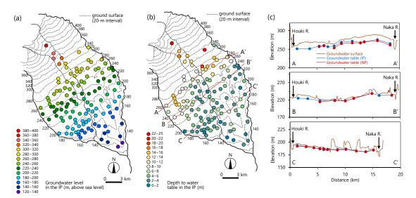
**Figure 3.** (a) Spatial distribution of the groundwater level in the irrigation period (IP), (b) depth to the water table in the IP, and (c) cross-sections of the groundwater table. The contour line of the ground surface was modified from the Geospatial Information Authority of Japan [30].
