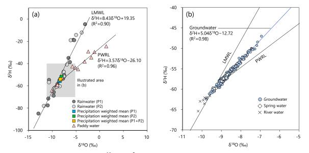
**Figure 8.** Relationship between  $\delta^{18}$ O and  $\delta^{2}$ H of (**a**) rainwater and paddy water and (**b**) groundwater. LMWL is the local meteoric water line identified by fitting a regression line to observations at sites P1 and P2. PWRL is the regression line fitted to the paddy water data.
