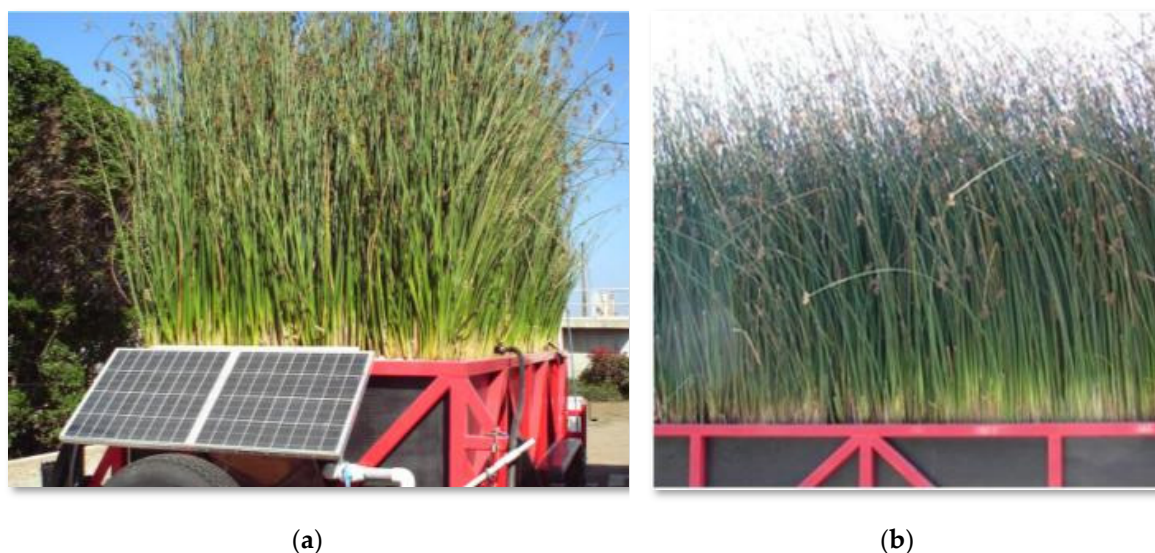
Figure 2. Pilot wetland system at the (a) beginning and (b) conclusion of the study. Note the high plant density and vigorous growth. Solar panels generated power for pumping water.
