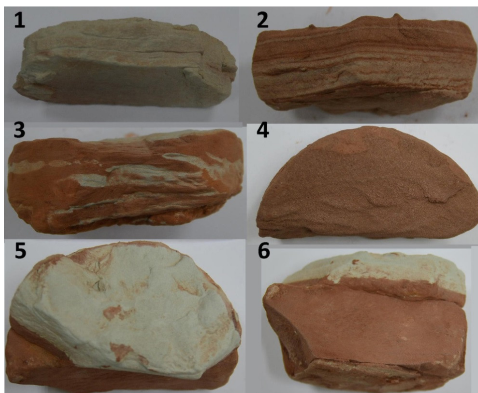
Figure 1. Photos of samples of studied rocks. 1—Green siltstones, 66.7–66.8 m. 2—Red sandstones, 75.2–75.3 m. 3—Variegated siltstones, 83.9–84 m. 4—Red siltstones, 94–94.1 m. 5–6—Green siltstones, 99.5–99.6 m (photo S. Druzhinin).
