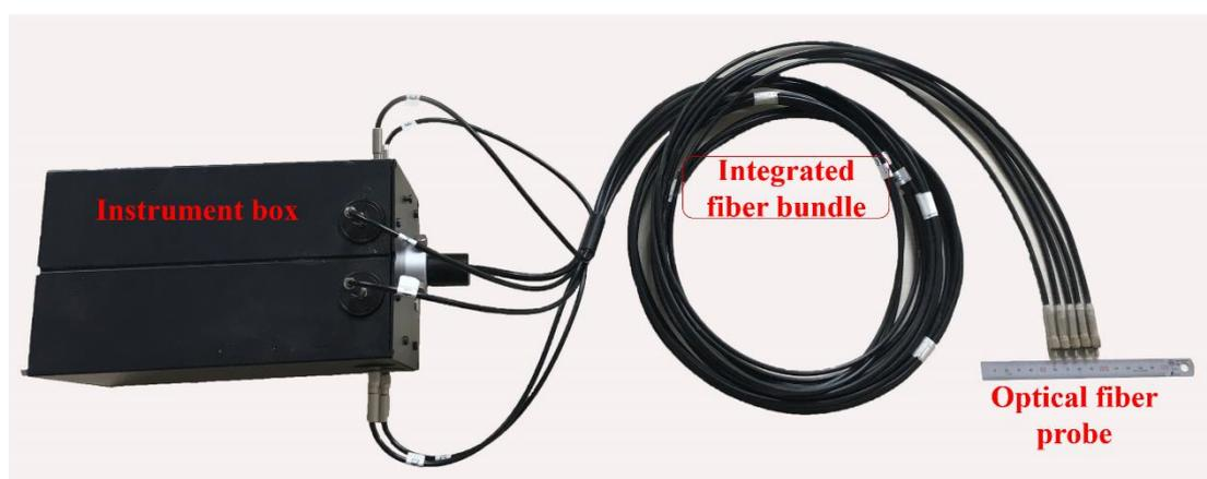
Figure 3. Five-channel optical fiber device for particle concentration measurement.
