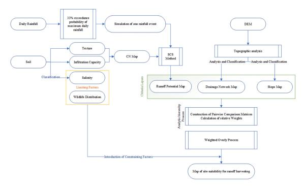
**Figure 3.** Flowchart illustrating the breakdown of the steps taken for identifying suitable areas for runoff harvesting in Kavir National Park.
