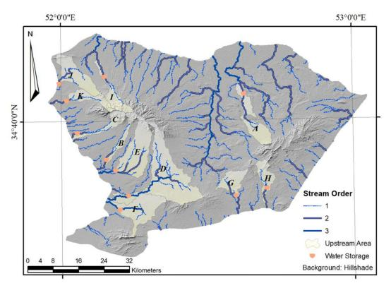
Figure 14. Possible locations for runoff harvesting structures in Kavir National Park.
