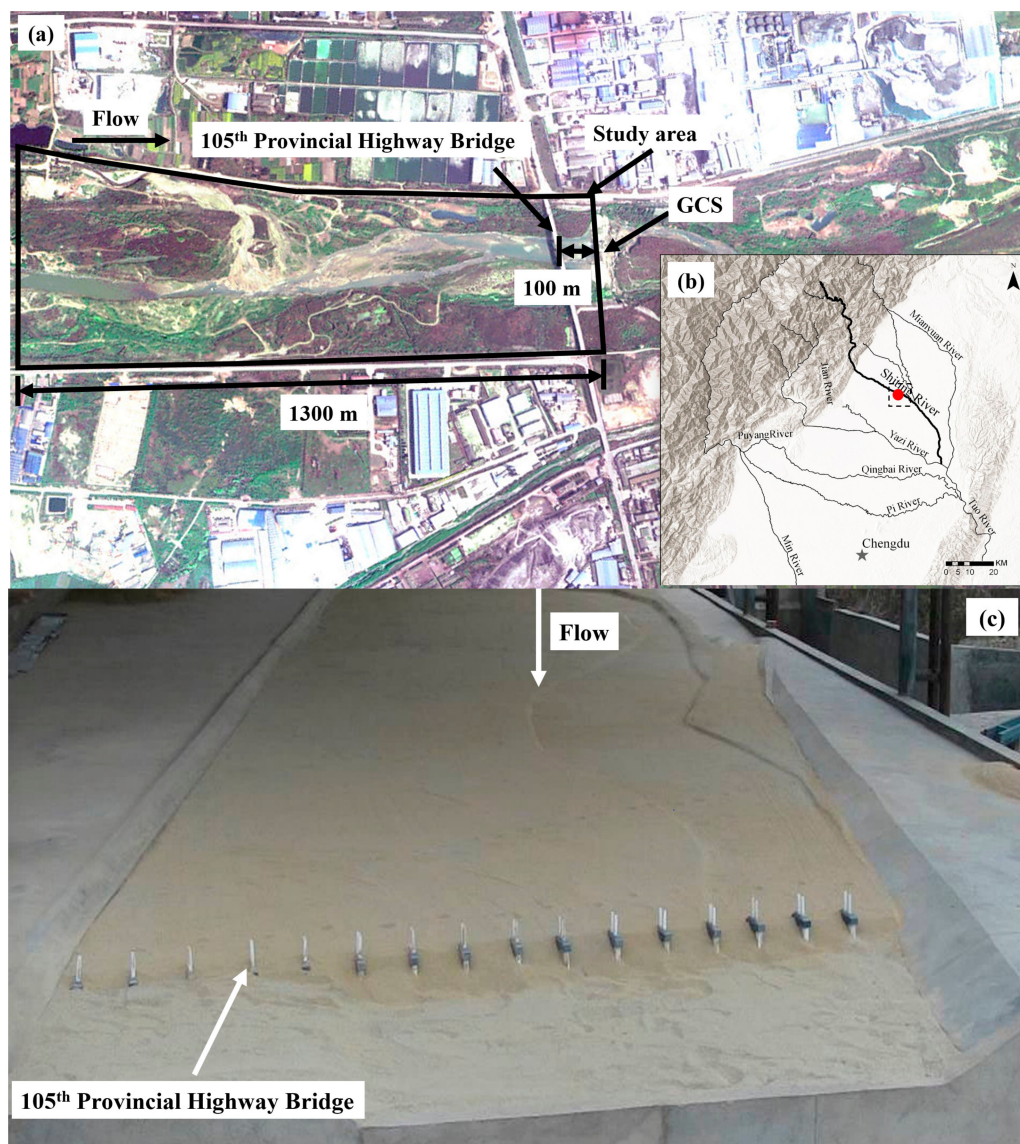
Figure 2. Plan view of the studied reach of Shiting River (a); location of Shiting River (b); a photo of the model (c).
