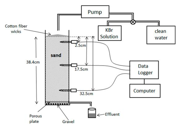
Figure 1. Schematic of the laboratory infiltration experimental setup.
