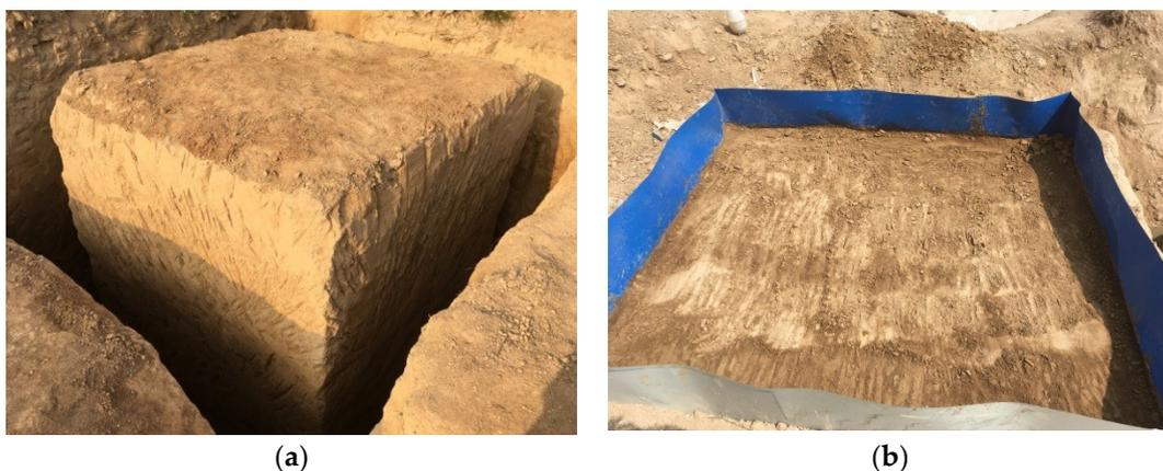
**Figure 2.** Field infiltration experiment: (a) the field soil column; (b) water retaining plate at the surface of the soil column.
