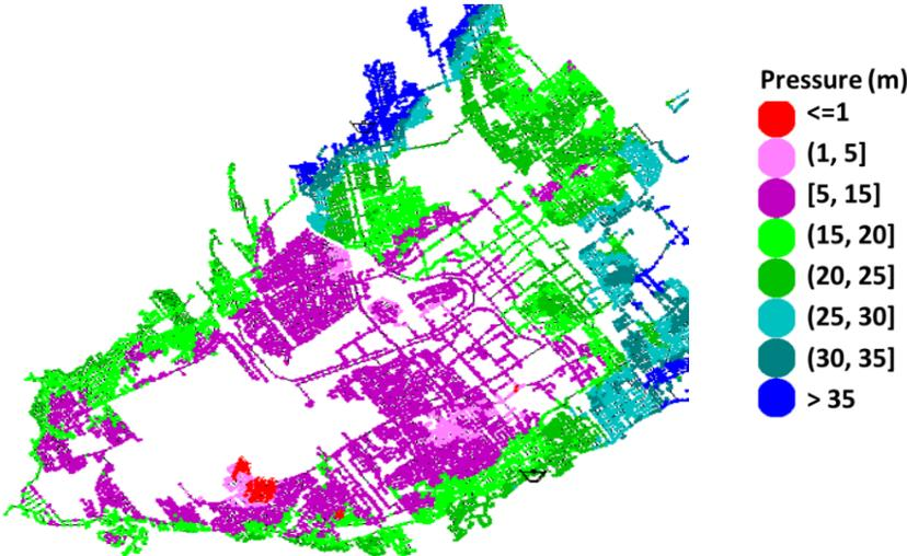
Figure S4. Spatial distribution of pressure using PDA under low/negative pressure event, at 7:00 PM.
