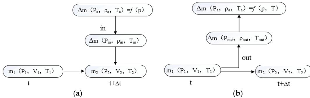
**Figure 2.** Processes of air passing through the air valve: (a) Gas sucking in; (b) gas discharging out.
