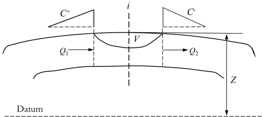
Figure 1. Schematic diagram of an air valve.
