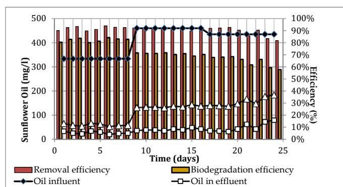
**Figure 5.** Changes in removal and biodegradation efficiencies of sunflower oil for the bench-scale activated sludge reactor.
