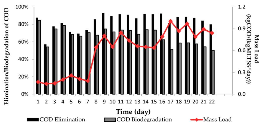
**Figure 7.** The efficiency of biodegradation and elimination as a function of mass loading in the experimental plant.
