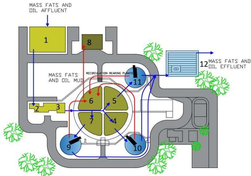
**Figure 2.** The wastewater treatment plant (WWTP) in this study. 1: Wastewater elevating plant. 2: Sedimentation tank. 3: Skimmer/degreaser. 4,5,7: Reactors. 6: Aerobic digester. 8: Band filter. 9,10,11: Clarifiers. 12: Contact camera.
