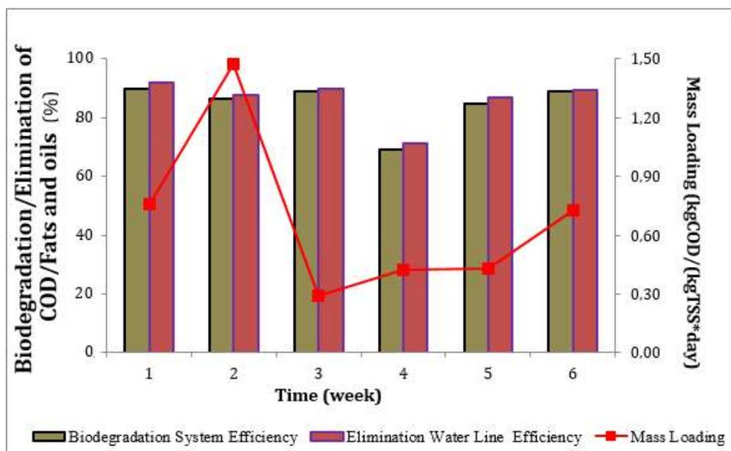
**Figure 8.** The efficiency of biodegradation and elimination of COD/fats and oils as a function of the mass loading in a WWTP-LA.
