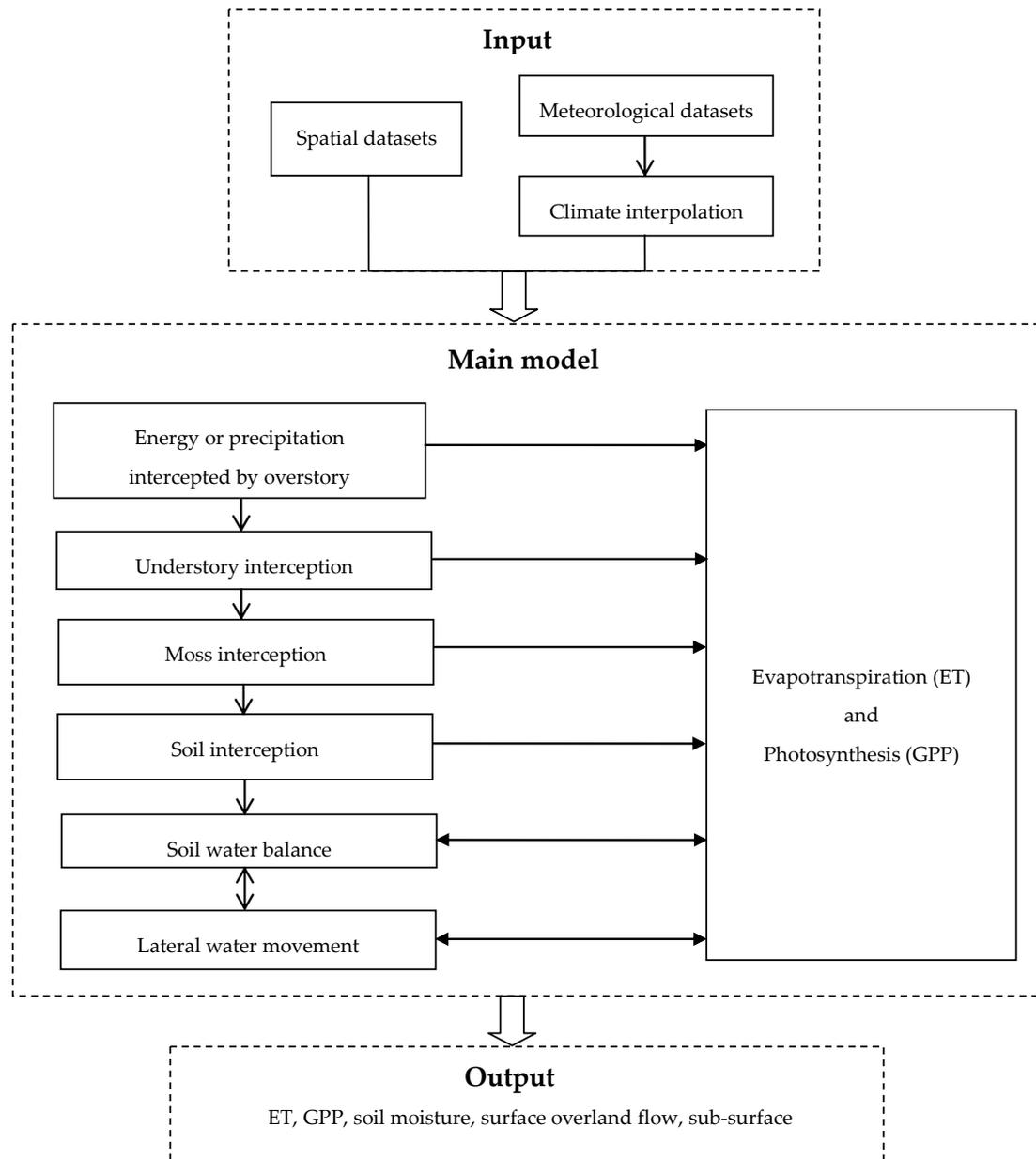
**Figure 2.** Flow chart of the DLM-Ecohydro model.
