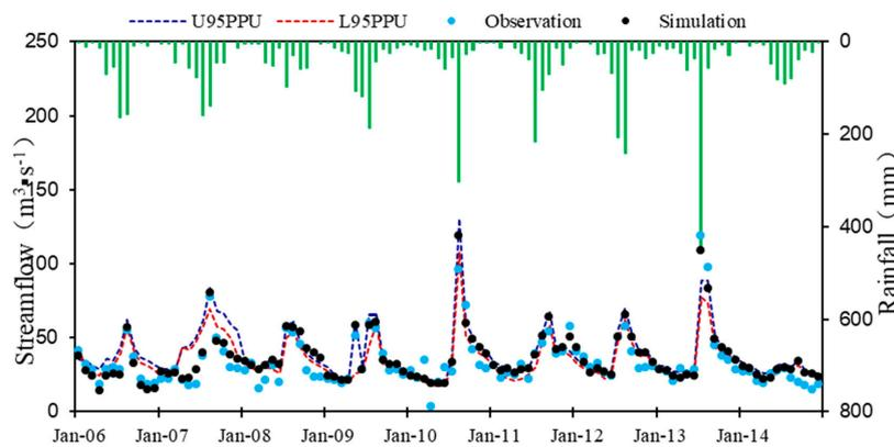
**Figure 4.** Runoff simulation of the Xiaoqing River basin in calibration and validation periods 95PPU based on SUFI-2.
