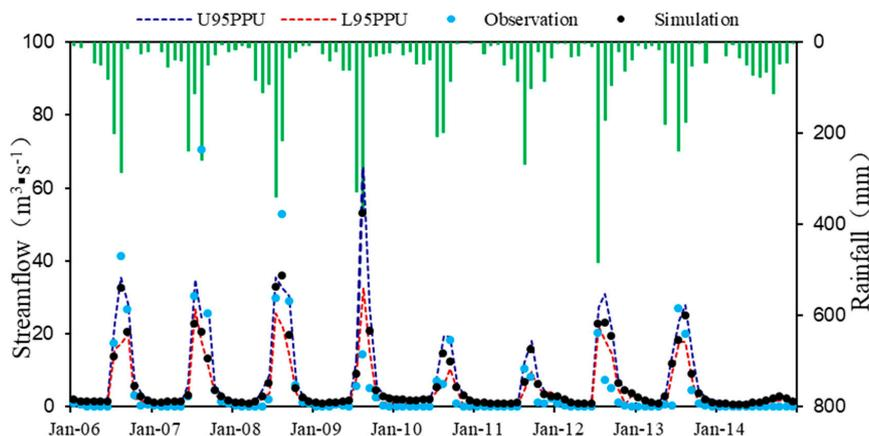
**Figure 8.** Runoff simulation of the Xinxue River basin in calibration and validation periods 95PPU based on SUFI-2.
