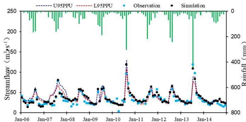
**Figure 5.** Runoff simulation of Xiaoqing River basin in calibration and validation periods 95PPU based on GLUE.
