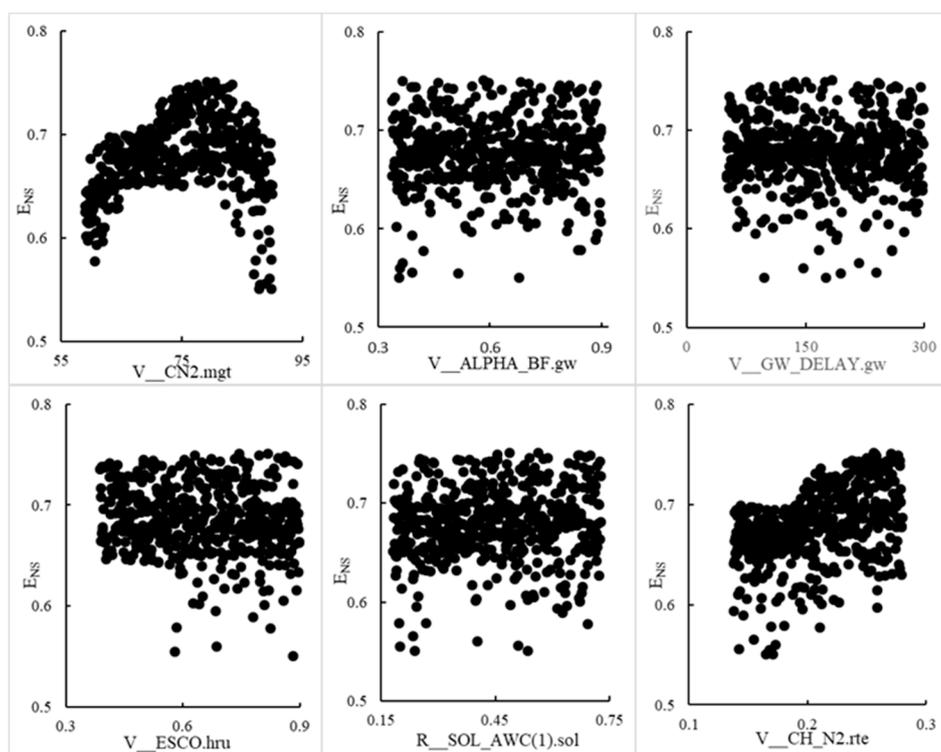
**Figure 6.** Parameter combination and distribution of Nash–Sutcliffe efficiency coefficient of Xinxue River basin based on SUFI-2.
