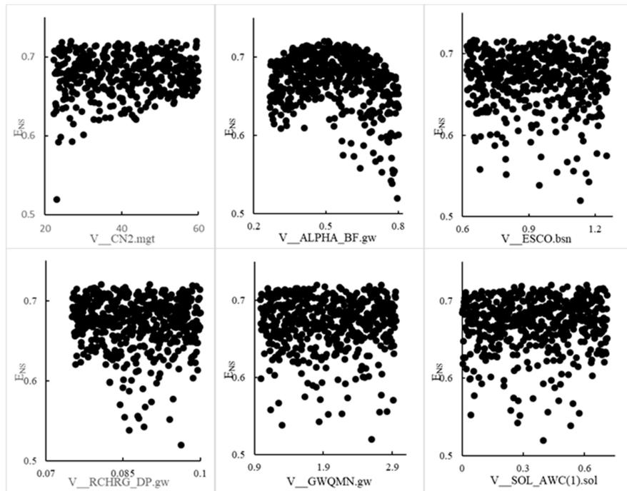
**Figure 2.** Parameter combination and Nash–Sutcliffe efficiency coefficient distribution diagram of the Xiaoqing River basin based on the SUFI-2 method.
