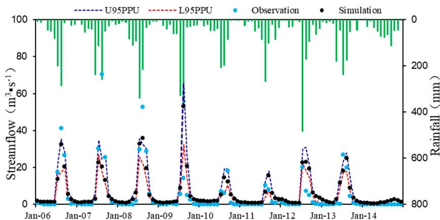
**Figure 9.** Runoff simulation of the Xinxue River basin in calibration and validation periods 95PPU based on GLUE.
