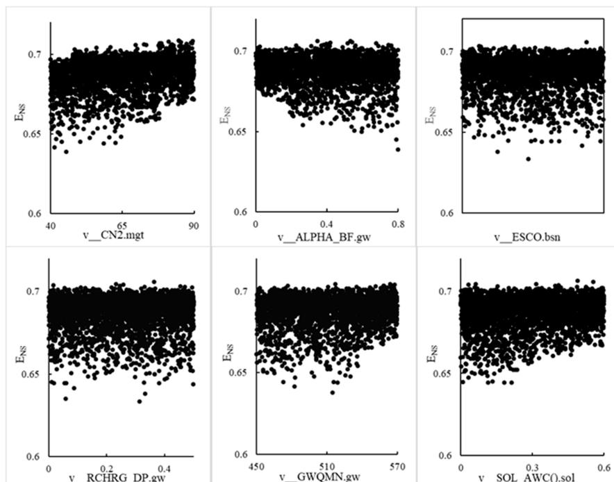
**Figure 3.** Parameter combination and Nash–Sutcliffe efficiency coefficient distribution diagram of the Xiaoqing River basin based on the GLUE method.
