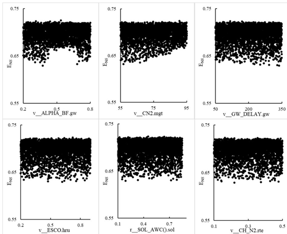
**Figure 7.** Parameter combination and distribution of Nash–Sutcliffe efficiency coefficient of Xinxue River basin based on GLUE.
