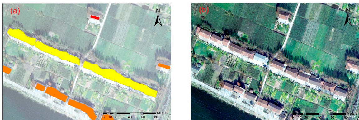
Figure 14. Example of adjoining buildings. (a) is vector data of buildings and (b) is remote sensing image of buildings.
